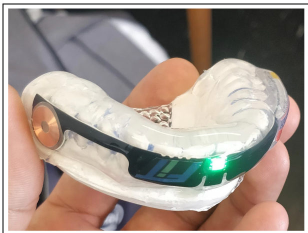
Figure 1. Instrumented mouthguard developed by Force Impact Technologies (FIT), used in this research.
