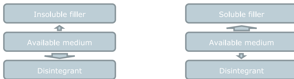
Fig. 8. Illustration of the competition-for-water hypothesis for a mixture of disintegrant with an insoluble, hydrophilic filler and a mixture of disintegrant with a soluble, hydrophilic filler.
