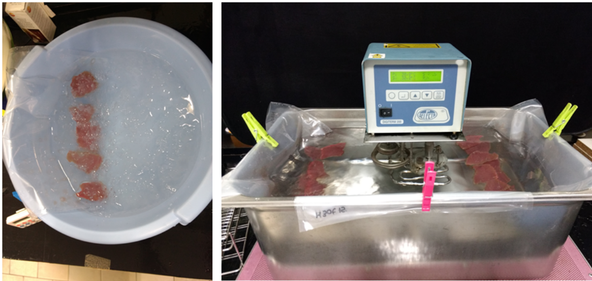
Figura 3.2: Meat water holding capacity test process.
