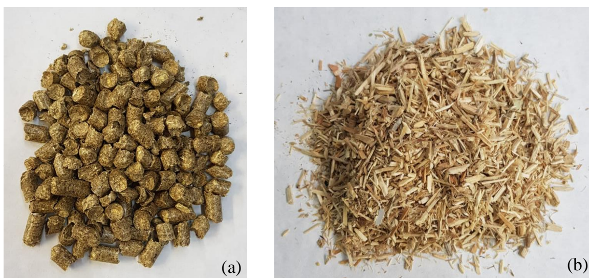
Figure 4. Biomass feedstock employed in this work: (a) wheat straw pellets and (b) untreated wood waste.
