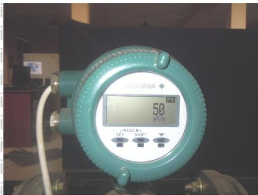
Gambar 4.3 Flow meter digital
