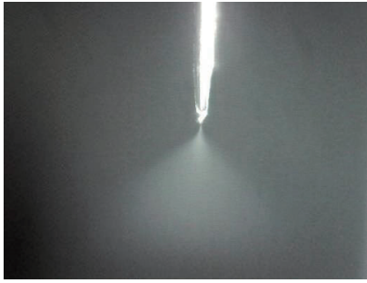
a) Electrospray without cell
