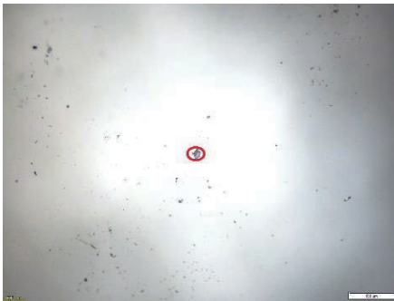
Fig.2 Optical micrograph of the ITO glass after electrospray.
