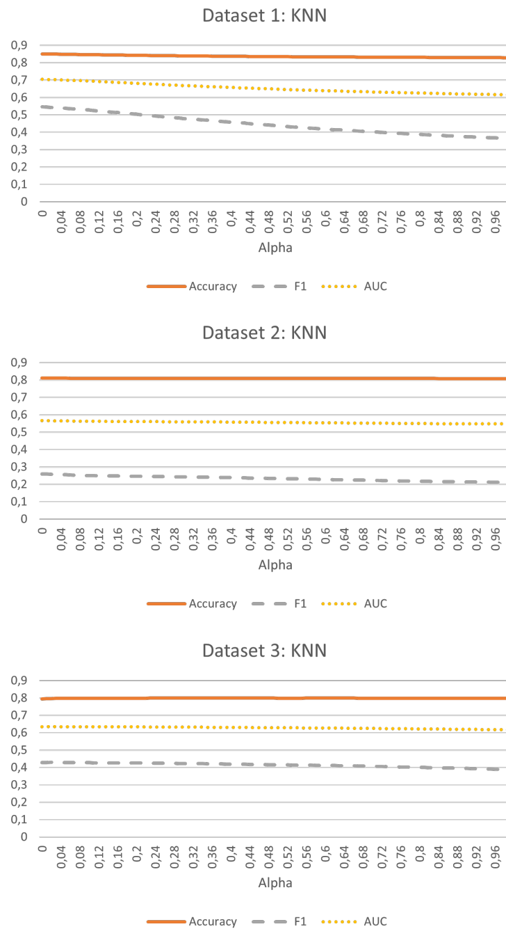
Figure 2.4: The accuracy, F1 and AUC values after noise insertion for all possible values of alpha as predicted by a k-nearest neighbour classifier on dataset 1, 2 and 3.
