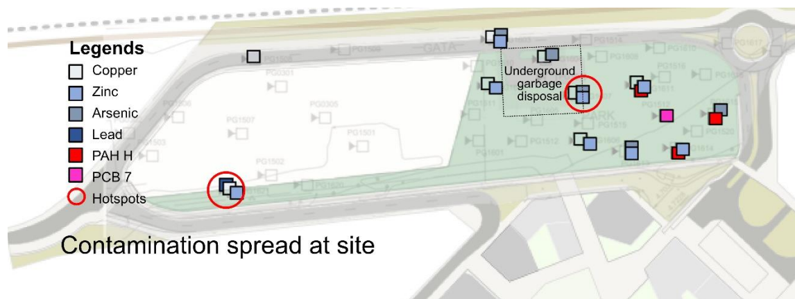
Figure 6: Spread of contamination across the site based on the SWECO report (Kaltin and Almqvist, 2016), the hotspots are circled red.
