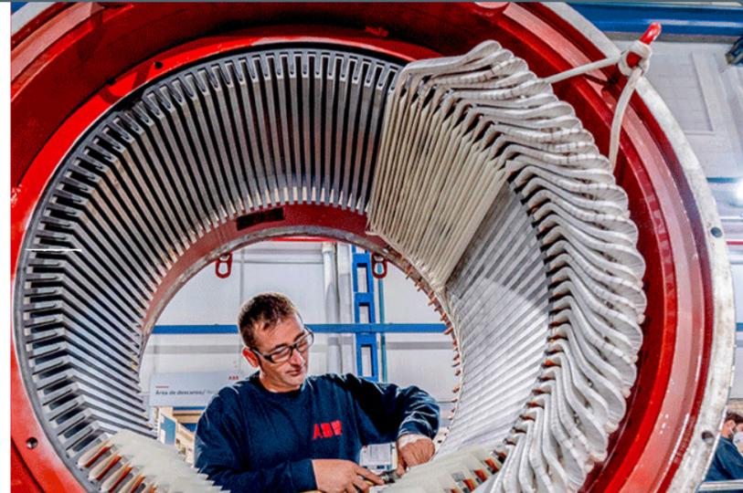
High voltage motors are often used until failure, with one of the most common faults occurring in the stator copper windings.
