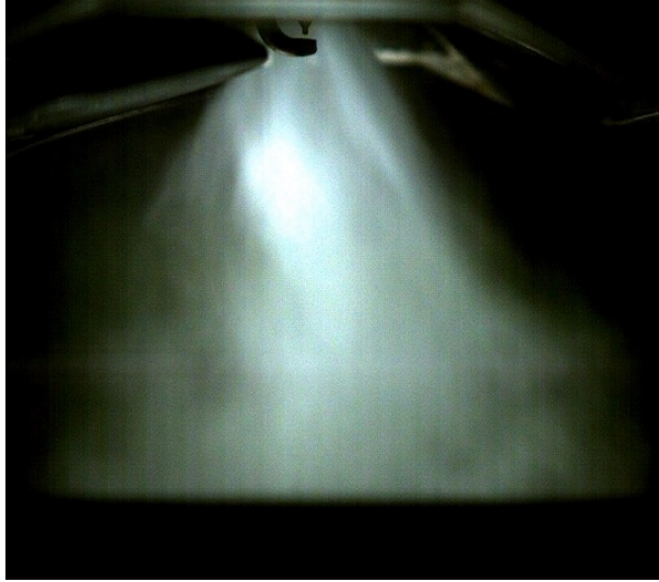
Figure 2.3: Image of a fuel spray injected into the cylinder of a GDI engine (SOI: -320 bTDC)
