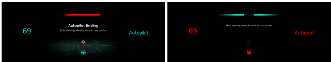
Figure 3. The instrument cluster view of the TOR (left) and the deactivation of AD (right), when the two steering wheel buttons are being pressed.
