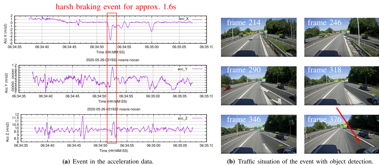
Fig. 2 Event where the truck was forced to conduct an unintended deceleration maneuver; no collision happened
