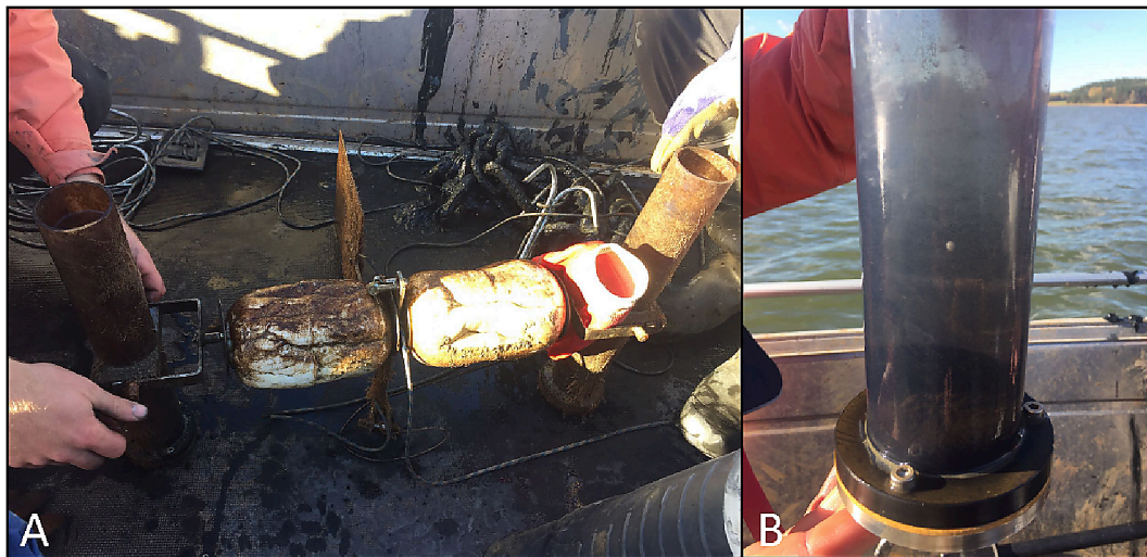
Fig. 3. Two funnel sediment trap with floaters (A) and a funnel containing sediment sample (B) after a trapping period.
