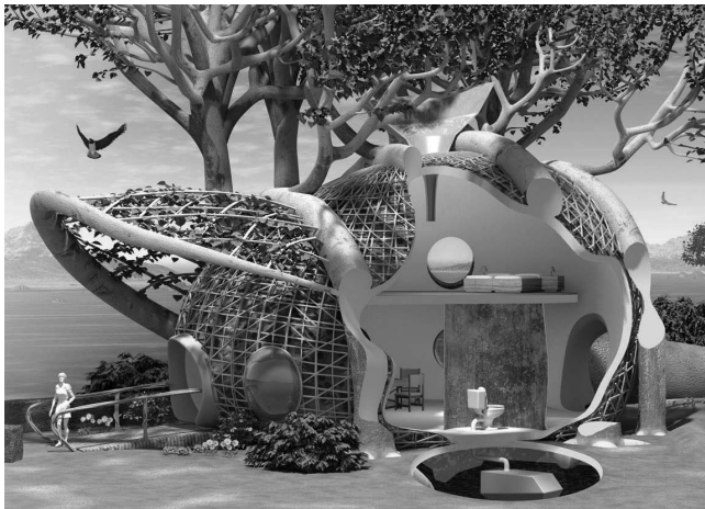
Figure 4. MIT Fab Tree Hab House has a living tree as the supporting structure – building itself as a living organism (Mawani, 2011. Courtesy by Joachim Mitchell).
