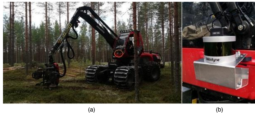
Figure 2. (a) Komatsu Forest 931.1 forest harvester. The lidar scanner is marked by a red circle in the front of the windshield of the cabin. (b) A close-up of the lidar scanner.
