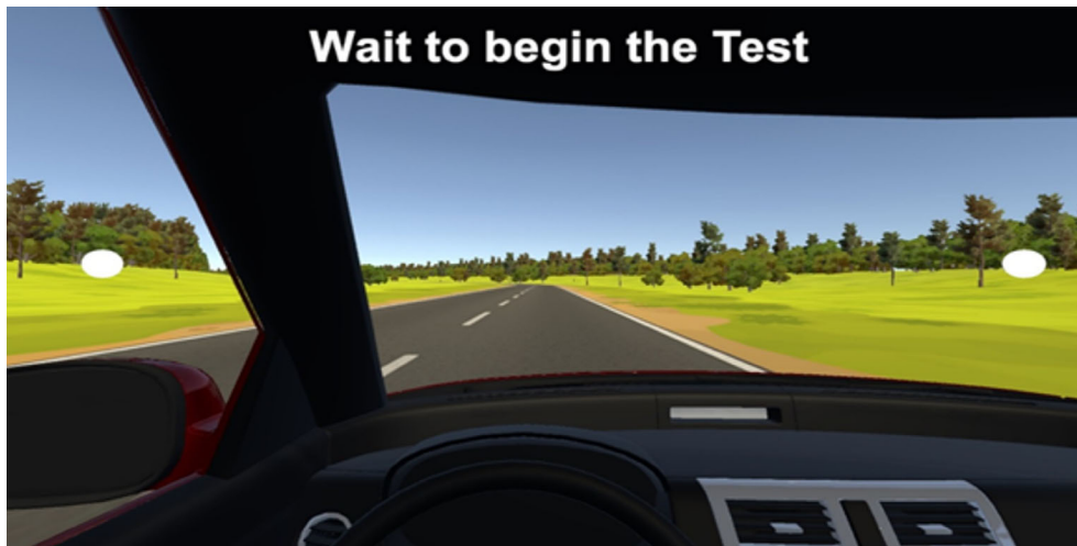
Fig. 1. The virtual driving car and scenery with white light spots flashed in the periphery used as visual stimuli.
