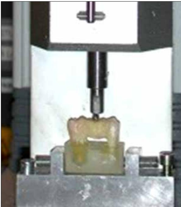
**Figure 3.** Placement of the steel ball to occlusal fossa.
