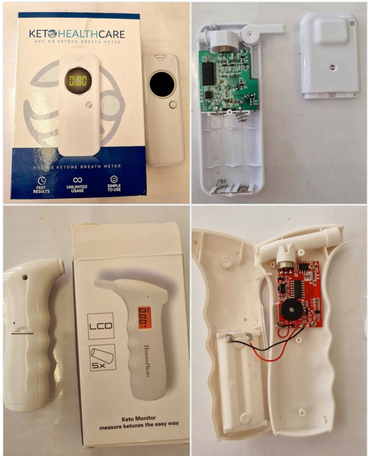
Fig 1. Tested breath ketone sensor devices. Note. The size of the required AA batteries displays the sensor sizes in the images of unassembled sensors.
