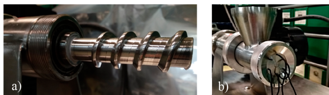
Figure 3. Photos of the extruder: (a) screw; (b) shaping of Pt catalyst.
