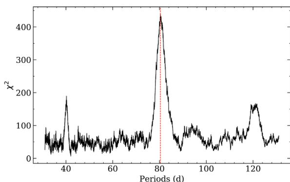
**Figure 8.**  $\chi^2$ s of fitting folded *RXTE/ASM* light curves (during the active period) to constants calculated by *efsearch* versus the periods used for folding. The best period found by *efsearch* is indicated with a dashed red line.
