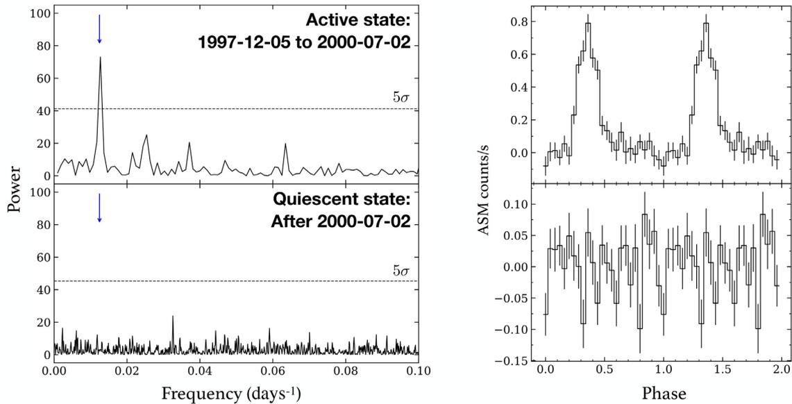
**Figure 9.** *Left:* ASM power spectra calculated with data from the active epoch (top) and data from the quiescent epoch (bottom). The dashed line in each panel depicts the  $5\sigma$  level. The best period ( $\approx 80.393$  d) is indicated with a blue arrow. *Right:* Corresponding light curves folded at the best period found by *efsearch*.
