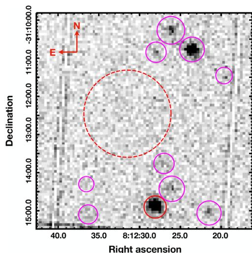
**Figure 2.** 0.5–7 keV X-ray image from the EPIC-PN camera on *XMM-Newton*. The image is 340 arcsec  $\times$  340 arcsec across. The source extraction region for J0812 is indicated with a solid red circle. The background region for extraction is indicated with a dashed red circle. Other nearby sources are indicated with solid magenta circles.
