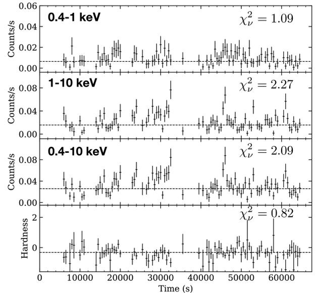
**Figure 6.** Time series rebinned to 500 s time bins. Light curves in soft (0.4–1.0 keV), hard (1–10 keV), and broad (0.4–10 keV) are shown in the first, second, and third panels, respectively. The bottom panel presents the time series of the hardness ratio defined by equation (1). Errors in the hardness ratio are propagated from errors in the soft and hard count rates. The dashed line in each panel marks the best-fitting constant.
