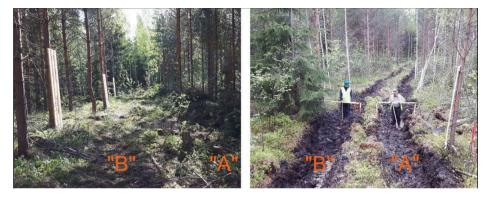
Figure 3. Start and end points of the test sites were marked with a detectable structure made of boards (left). The depths of both ruts ("A" & "B") were manually measured at 1-m intervals with a horizontal hurdle and measuring rod.
