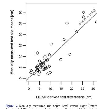
Figure 7. Manually measured rut depth [cm] versus Light Detection and Ranging (LiDAR)-derived rut depth and the linear model fitted to the data (gray line).
