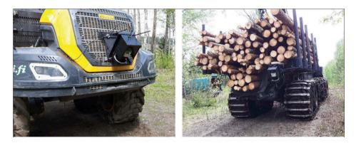
Figure 2. The 2D Light Detection and Ranging (LiDAR) sensor mounted on the rear of the Ponsse Scorpion King harvester (left) and on the Ponsse Elk forwarder (right).
