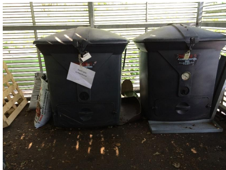
Figure 5. Biolan Quick Composters 550-L in the waste collection points. The note informs the staff which composter is currently being filled. Photo by Leena Erälinna.
