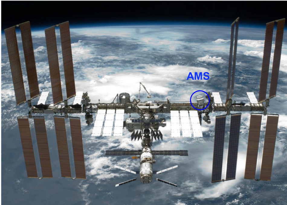
Fig. 1. AMS is a unique precision magnetic spectrometer on the ISS. AMS will operate on the ISS for the Station's lifetime. It is mounted on the ISS with a 12 degree angle to the zenith to prevent that the rotating ISS solar arrays are in the AMS field of view.
