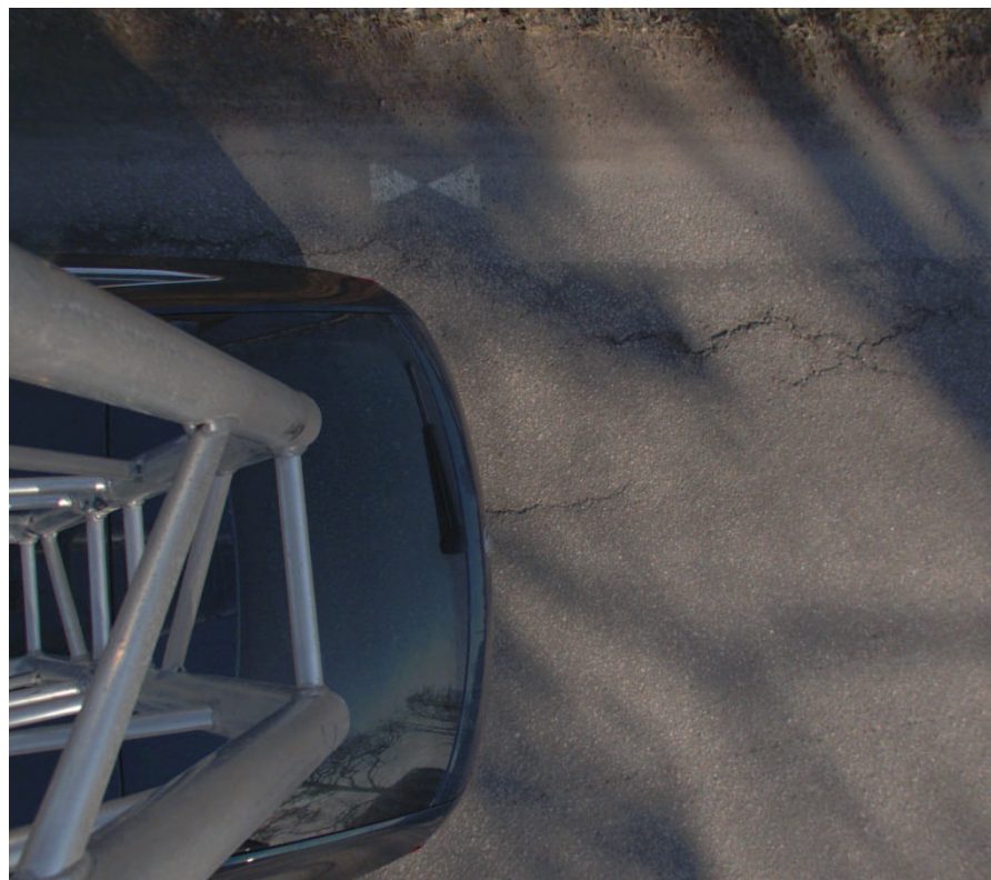
Figure 2. Ground target painted on the pavement. The location for the target was measured to the center between the two triangles.
