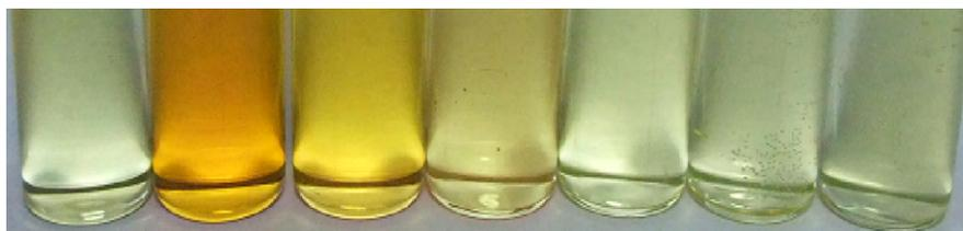
**Fig. 3.** Color changes of the sensor **1** in 9/1 DMSO/H<sub>2</sub>O (v/v) in absence and presence of anions (from the left to right: **1** only, **1** + AcO<sup>-</sup>, **1** + F<sup>-</sup>, **1** + H<sub>2</sub>PO<sub>4</sub><sup>-</sup>, **1** + Cl<sup>-</sup>, **1** + Br<sup>-</sup> and **1** + I<sup>-</sup>).
