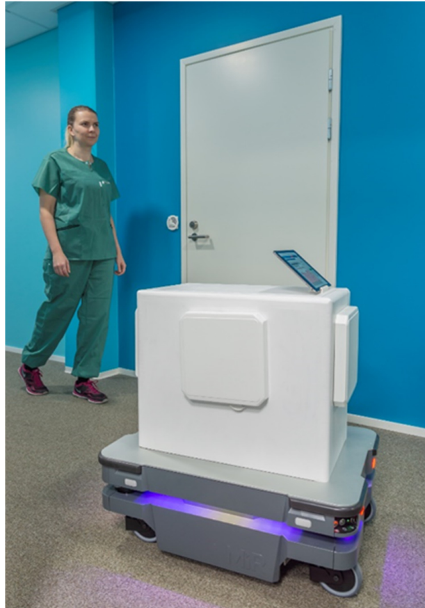
Figure 2. In the orientation work, the mobile robot meets and identifies the caregiver based on the RFID tags on her shirt.
