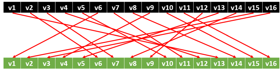
Fig. 2 The pattern of the Led-Pattern. Herein, v_1, v_2, \dots, v_{16} define values of the used overlapping block with a length of 16
