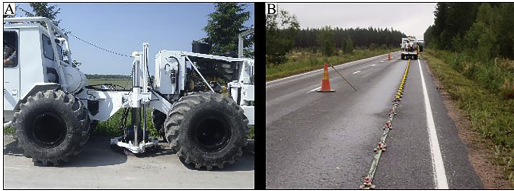
Fig. 3. a) IVI Minivib (Geological Survey of Canada). b) The 200 m landstreamer with 3-component (yellow) and vertical component geophones (red) (COWI Denmark). Photos by Elina Ahokangas, Fig. 3a taken 31.5.2011 and Fig. 3b 2.9.2011.
