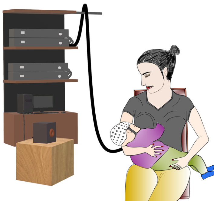
Fig 2. Schematic illustration of near-infrared spectroscopy experimental setup. The parent can hold the baby on her lap during the measurement.
