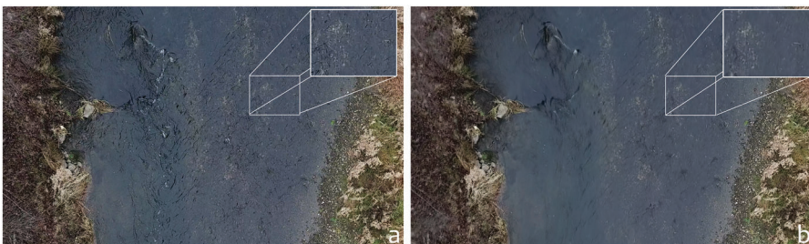
FIGURE 3 Example of the difference between original head frame and filtered median frame processed after tailing frames had been co-registered to the head frame
