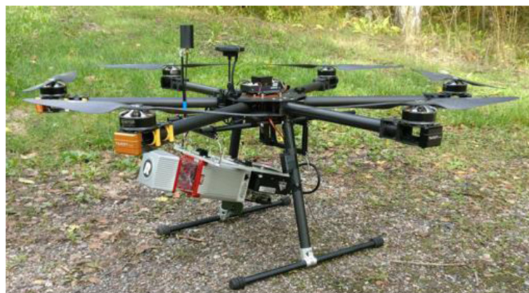
Fig. 2 The ULS system, including the drone, the scanner, and the GNSS-IMU
