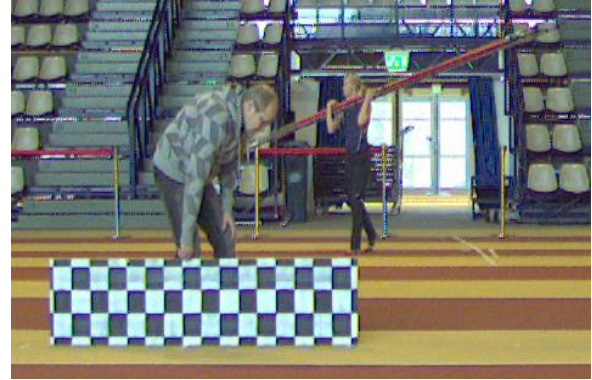
Figure 3. Calibration chessboard at the projection plane
