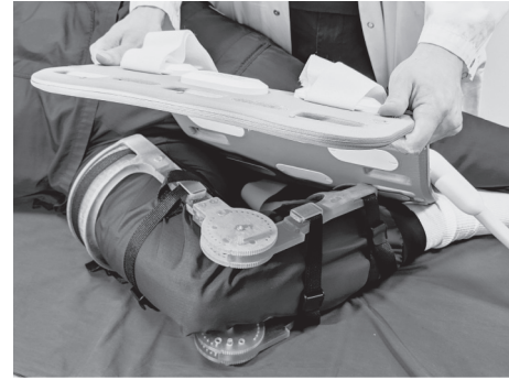
FIGURE 1: Positioning of the bent knee for the MRI scan with the in-house MRI-compatible 3D-printed knee brace. The 18-channel body matrix coil was placed over the knee joint.
