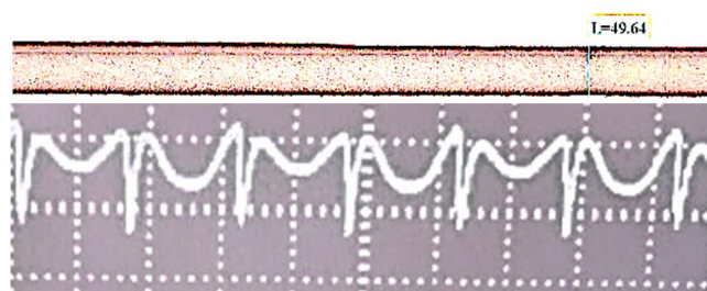
FIGURE 21. Scribe thickness of 49.64 \mu and oscilloscope measurement.
