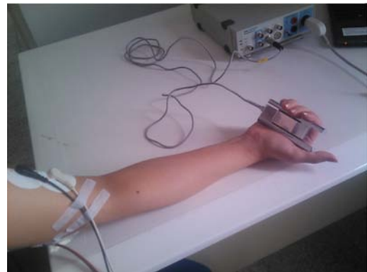
Fig. 1: Bipolar surface electromyographic electrode placement over the biceps brachii muscle.
