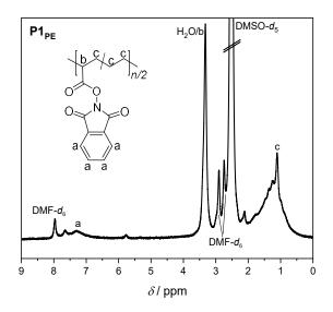
**Figure 53**: <sup>1</sup>H NMR spectrum of **P1**<sub>PE</sub> after thermally-induced decarboxylation. Solvent: 50:50 mixture of DMF- $d_7$  and DMSO- $d_6$ .
