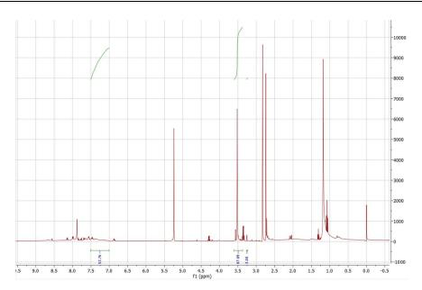
**Figure 73**: <sup>1</sup>H NMR of **DP2**<sub>PE</sub> after decarboxylation with additional *i*-PrOH. Integrals of relevant signals at 3.25 ppm, 3.51 ppm, and 7.35 ppm for the calculation of the improvement of the decarboxylation result are marked.
