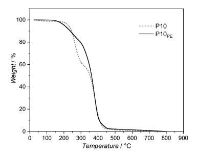
**Figure 66**: Thermogravimetrical analysis of **P10**<sub>PE</sub> in comparison to **P10**, heating rate 10 K min<sup>-1</sup>.
