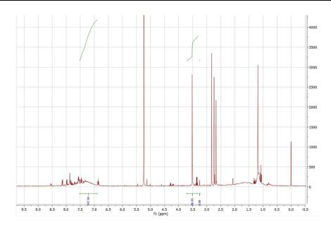
**Figure 71**: <sup>1</sup>H NMR of **DP2**<sub>PE</sub> after decarboxylation with reduced equivalents of phenylsilane. Integrals of relevant signals at 3.25 ppm, 3.51 ppm, and 7.35 ppm for the calculation of the improvement of the decarboxylation result are marked.
