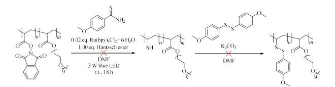
Scheme 42: Decarboxylative thiolation of FP2 with 4-methoxythiobenzamide followed by functionalization with bis-(4-methoxyphenyl)disulfide.
