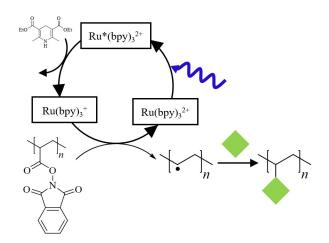
Scheme 39: Functionalization of PAP *via* photochemical decarboxylation using the carboncentered radical formed at the polymer backbone.
