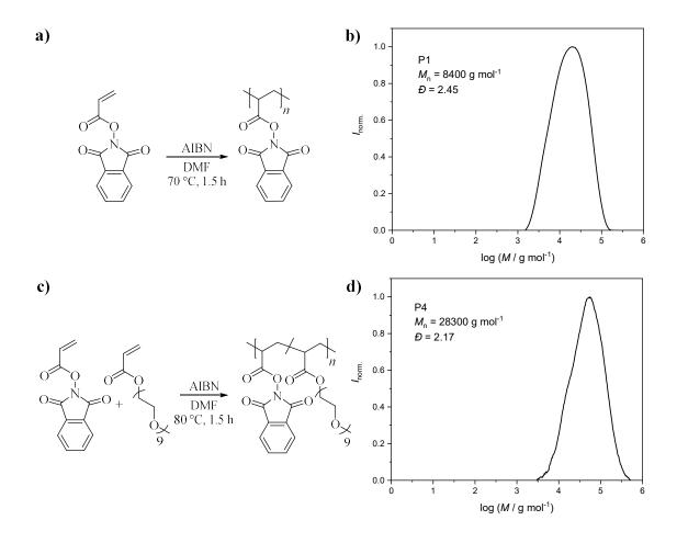
**Figure 2**: **a)** Polymerization of NAP to PAP and the analysis of PAP (P1) by **b**) SEC with DMAc as eluent and PMMA calibration. **c)** Copolymerization of NAP with OEGMEA yielding P[AP-*co*-OEGMEA] (P4) and **d)** the corresponding SEC chromatogram in DMAc as eluent using PMMA calibration.
