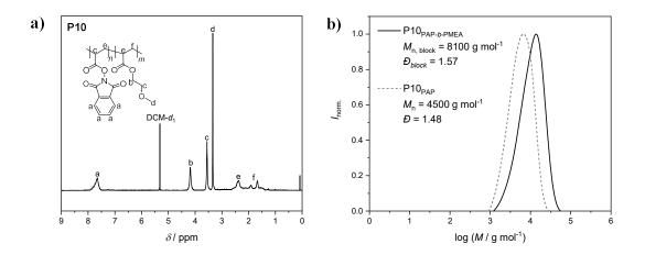
**Figure 6**: a) <sup>1</sup>H NMR spectrum of PAP-*b*-PMEA (**P10**) and b) the corresponding SEC chromatogram in DMAc as eluent with PMMA calibration.
