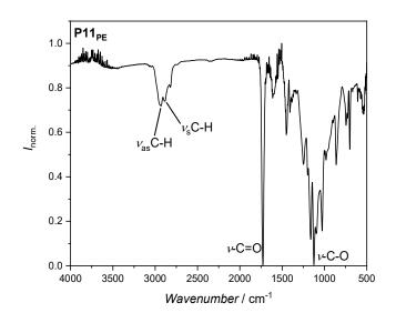
Figure 68: ATR-FT-IR spectrum of P11<sub>PE</sub> (PE-*b*-PMEA) after thermal decarboxylation.
