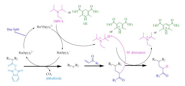
**Scheme 22**: Mechanism of the photochemical decarboxylation of *N*-(acyloxy)phthalimide with  $Ru(bpy)_3Cl_2 \cdot 6 H_2O$  as metal catalyst, HE (green) or DIPEA (purple) as reductant and radical quencher and the electron-deficient alkene (Michael-acceptor, blue).<sup>115</sup>
