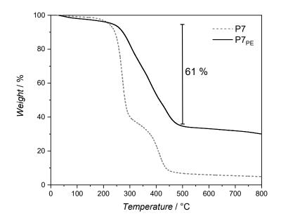
Figure 63: Thermogravimetrical analysis of  $P7_{PE}$  in comparison to P7, heating rate 10 K min<sup>-1</sup>.
