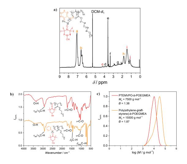
**Figure 42**: a) <sup>1</sup>H NMR spectrum of **poly(ethylene-***graft***-styrene)**-*b***-POEGMEA**. b) Comparison of the ATR-FT-IR spectra of **PTEMVPO**-*b***-POEGMEA** (top, red) and **poly(ethylene-***graft***-styrene)**-*b***-POEGMEA** (bottom, orange) and c) comparison of the SEC chromatogram before (red) and after grafting of styrene (orange) in DMAc as eluent and PMMA calibration.
