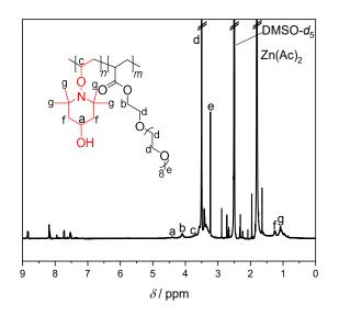
**Figure 80**: <sup>1</sup>H NMR spectrum of **PTEMVPO-***b***-POEGMEA** after reduction with Zn/AcOH in DMF at 60 °C; solvent: DMSO-*d*<sub>6</sub>.
