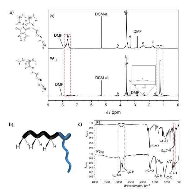
**Figure 9**: a) <sup>1</sup>H NMR spectra of PAP-*b*-POEGMEA (P6) and PE-*b*-POEGMEA (P6<sub>PE</sub>) after photochemically-induced decarboxylation, b) schematic depiction of the block ratios of block copolymer P6<sub>PE</sub>, with PE (black) and POEGMEA (blue) blocks and c) comparison of the ATR-FT-IR spectra before (top) and after (bottom) photochemically-induced decarboxylation.
