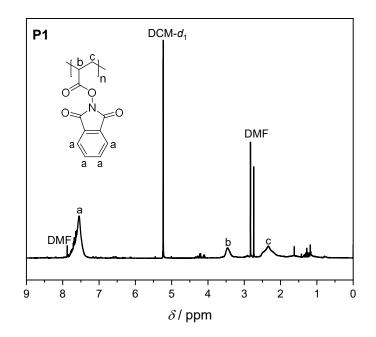
Figure 52: <sup>1</sup>H NMR spectrum of PAP (P1). Solvent DCM-*d*<sub>2</sub>.
