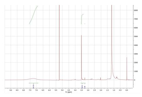
**Figure 70**: <sup>1</sup>H NMR spectrum (raw spectrum) of **DP2**<sub>PE</sub> after decarboxylation under standard conditions (1.50 eq. phenylsilane). The integrals of relevant signals at 3.25 ppm, 3.51 ppm, and 7.35 ppm for the calculation of the improvement of the decarboxylation result are marked.
