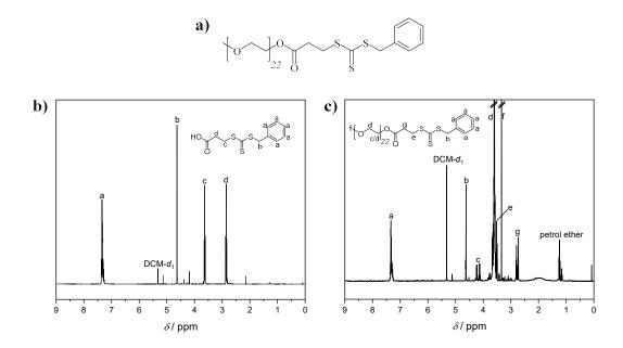
**Figure 16**: **a)** Structure of the macroRAFT-agent BTTP-mPEG<sub>1000</sub> and the <sup>1</sup>H NMR spectra of **b)** BTTP and **c)** BTTP-mPEG<sub>1000</sub>.
