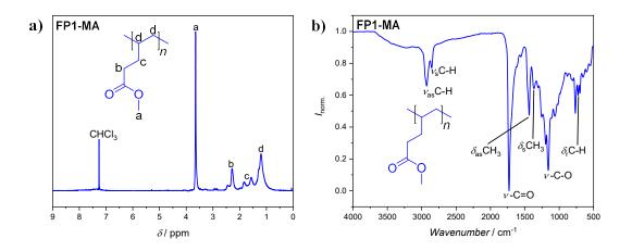
Figure 29: Analysis of FP1-MA via a) <sup>1</sup>H NMR spectroscopy and b) ATR-FT-IR spectroscopy.
