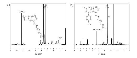
Figure 32: <sup>1</sup>H NMR spectra of a) the decarboxylative thiolation of FP2 with 4-methoxythiobenzamide and b) the following functionalization in a one-pot two-step process with bis-(4-methoxyphenyl)disulfide.
