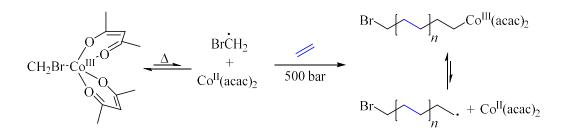
Scheme 11: Mechanism of the cobalt-mediated radical polymerization of ethylene demonstrated by Detrembleur *et al.*<sup>16</sup>
