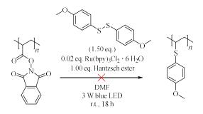
Scheme 41: Decarboxylative functionalization of FP1 with bis-(4-methoxyphenyl)disulfide.
