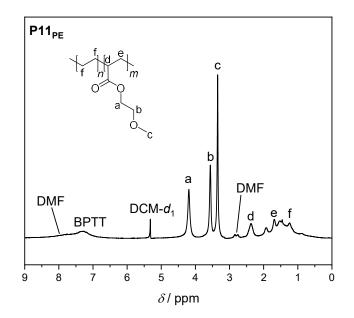
**Figure 67**: <sup>1</sup>H NMR spectrum of **P11**<sub>PE</sub> (PE-*b*-PMEA) after thermal decarboxylation. Solvent: DCM-*d*<sub>2</sub>.
