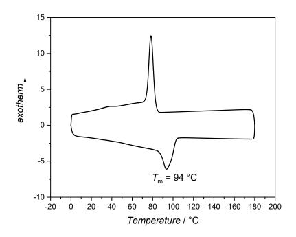
**Figure 76**: DSC analysis of commercial PE (Polyethylene, Sigma Aldrich, average  $M_n = 7700 \text{ g mol}^{-1}$ , 427799-250G).
