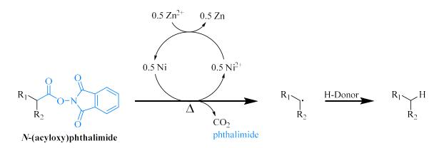
Scheme 23: Mechanism of the thermally-induced, nickel-catalyzed decarboxylation of N-(acyloxy)phthalimide as used in the present thesis with NiCl<sub>2</sub> as metal catalyst and zinc as reductant.<sup>125</sup>
