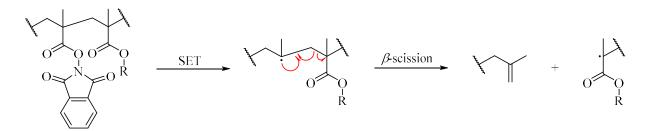
Scheme 52: Proposed mechanism of the SET-induced decarboxylative backbone degradation of PMAP copolymers by Sumerlin *et al.*<sup>155</sup>
