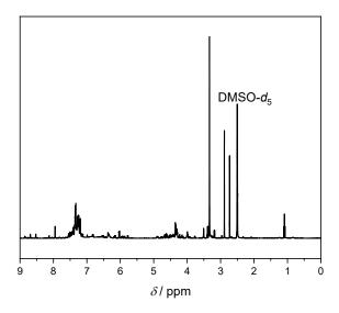
**Figure 89**: <sup>1</sup>H NMR spectrum of **PP1**<sub>PE</sub> after decarboxylation with Ru(bpy)<sub>3</sub>Cl<sub>2</sub> · 6 H<sub>2</sub>O, BNAH as reductant and Bu<sub>3</sub>SnH as H-donor. Solvent: DMSO- $d_6$ .
