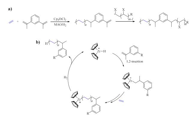
Scheme 12: a) Polymerization of ethylene using 1,3-diisopropenylbenzene (DIB),  $Cp_2ZrCl_2$  as catalyst, methylaluminoxane (MAO) as cocatalyst and hydrogen with the following block formation as demonstrated by Scott *et al.*<sup>61</sup> b) Simplified mechanism of the polymerization of ethylene with DIB and  $Cp_2ZrCl_2$ .<sup>61</sup>
