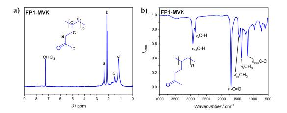
Figure 30: Analysis of FP1-MVK via a) <sup>1</sup>H NMR spectroscopy and b) ATR-FT-IR spectroscopy.
