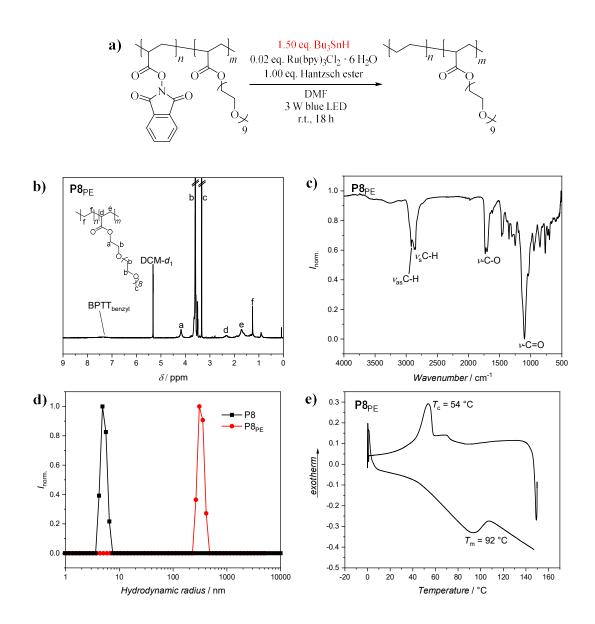
**Figure 12**: a) Photochemical decarboxylation of PAP-*b*-POEGMEA (**P8**) with tributyltin hydride and the analysis of **P8**<sub>PE</sub> via b) <sup>1</sup>H NMR spectroscopy, c) ATR-FT-IR spectroscopy, d) DLS and e) DSC revealing  $T_m = 92$  °C and  $T_c = 54$  °C.
