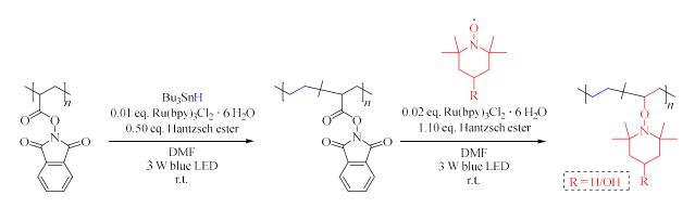
**Scheme 46**: Synthesis of poly(ethylene-*co*-TEMVP) from PAP *via* a two-step reaction with the partly reductive decarboxylation with Bu<sub>3</sub>SnH in the first step, followed by the decarboxylative functionalization with TEMPO.
