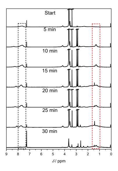
**Figure 65**: Reaction monitoring of thermally-induced decarboxylation of PAP-*b*-POEGMEA (P11). Solvent: CDCl<sub>3</sub>.
