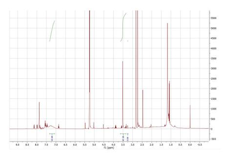
**Figure 74**: <sup>1</sup>H NMR of **DP2**<sub>PE</sub> after decarboxylation with reduced concentration and additional *i*-PrOH. Integrals of relevant signals at 3.25 ppm, 3.51 ppm, and 7.35 ppm for the calculation of the improvement of the decarboxylation result are marked.
