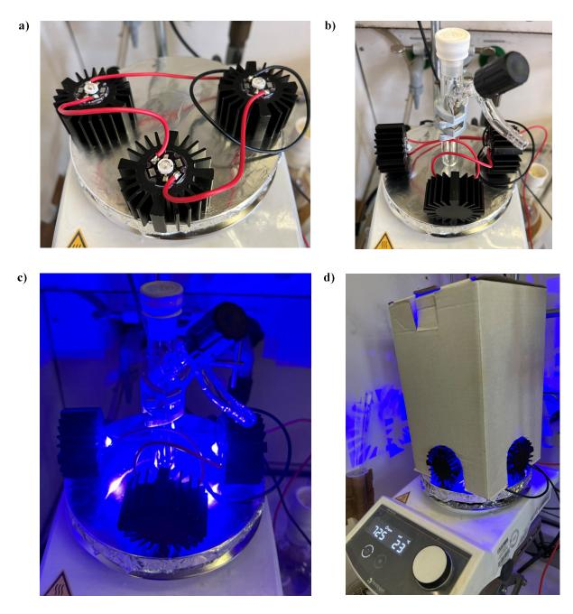
**Figure 51**: Photos of the LED setup used for photochemical reaction. **a**) Avonec 3 W high power LEDs on a star plate. **b**) LEDs with Schlenk tube used for the decarboxylation, placed in a distance of 1.5 cm around the tube. **c**) Schlenk tube with LEDs turned on. **d**) Final reaction setup with custom-build protection ensuring the removal of the heat produced by the LEDs.
