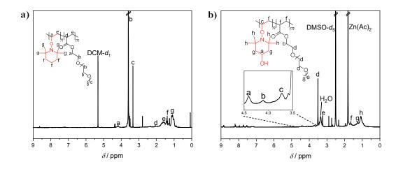
**Figure 40**: <sup>1</sup>H NMR spectra of reduction of **a**) **PTEMVP-***b***-POEGMEA** in DMF at 60 °C with Zn/AcOH (Table 5, entry #2) and b) PTEMVPO-*b***-POEGMEA** in DMF at 80 °C with Zn/AcOH (Table 5, entry #5).
