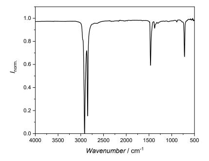
**Figure 75**: ATR-FT-IR spectrum of commercial PE (Polyethylene, Sigma Aldrich, average  $M_n = 7700 \text{ g mol}^{-1}$ , 427799-250G).
