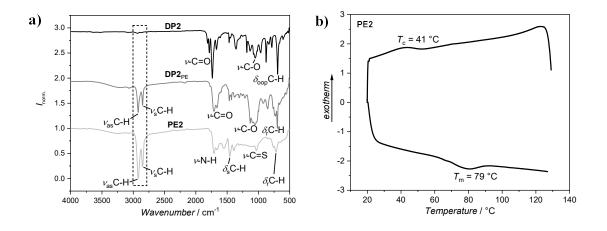
**Figure 19: a)** ATR-FT-IR spectra of the **DP2** precursor (top, black), after decarboxylation (**DP2**<sub>PE</sub>, middle, grey) and after cleavage (**PE2**, bottom, light grey). **b)** DSC chromatogram of **PE2** obtained after decarboxylation and cleavage of **DP2**.
