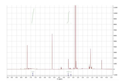
**Figure 72**: <sup>1</sup>H NMR of **DP2**<sub>PE</sub> after decarboxylation with reduced concentration. Integrals of relevant signals at 3.25 ppm, 3.51 ppm, and 7.35 ppm for the calculation of the improvement of the decarboxylation result are marked.
