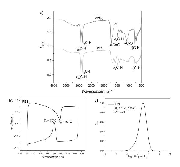
Figure 22: a) Comparison of the ATR-FT-IR spectra of  $DP3_{PE}$  before (top, black) and PE3 after (bottom, grey) cleavage with ethylenediamine at room temperature. Analysis of PE3 by b) DSC and c) HT-SEC in 1,2,4-TCB at 160 °C.
