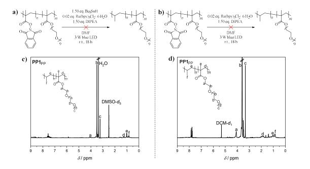
Figure 46: a) Decarboxylation of PP1 with  $Ru(bpy)_3Cl_2 \cdot 6H_2O$ , DIPEA as reductant, and Bu<sub>3</sub>SnH as H-donor in DMF as solvent and b) decarboxylation of PP1 with  $Ru(bpy)_3Cl_2 \cdot 6H_2O$  and DIPEA as reductant and H-donor in DMF as solvent as well as the corresponding analyses *via* c)/d) <sup>1</sup>H NMR spectroscopy.
