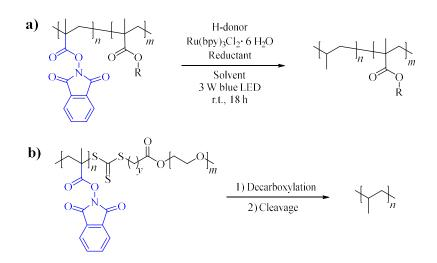
Scheme 49: Intended concept of the propylene-free synthesis of **a**) PP block copolymers and **b**) PP homopolymers from methacrylate-based precursor polymers by photochemical decarboxylation.
