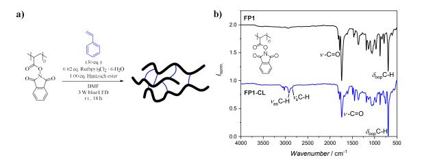
Figure 31: a) Side chain polymerization of styrene on FP1 in the absence of DIPEA and formation of a cross-linked polymer (FP1-CL). b) Comparison of ATR-FT-IR spectra of FP1 (PAP) (top, black) with FP1-CL (bottom, blue).
