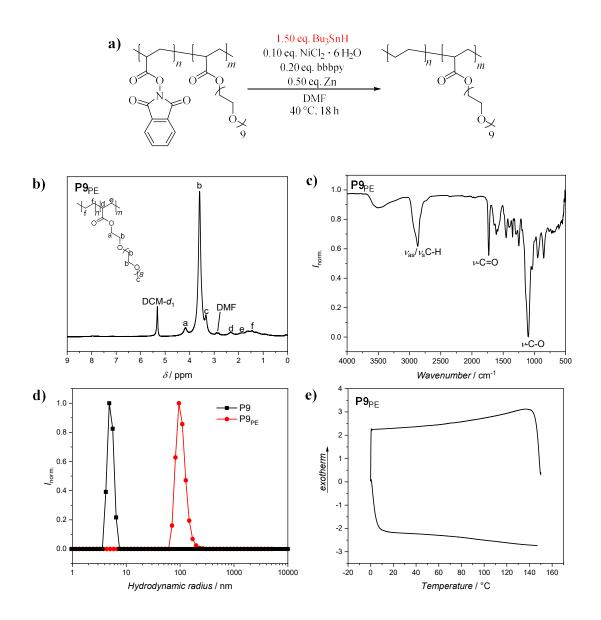
**Figure 13**: **a)** Thermal decarboxylation of **P9** with tributyltin hydride and the analysis of **P9**<sub>PE</sub> *via* **b)** <sup>1</sup>H NMR spectroscopy, **c)** ATR-FT-IR spectroscopy, **d)** DLS, and **e)** DSC, which did not reveal a melting or crystallization of the material.
