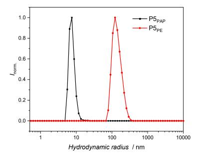
Figure 60: DLS analysis of P5 and P5<sub>PE</sub> after photochemically-induced decarboxylation with phenylsilane.
