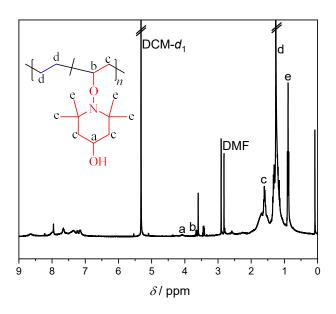
**Figure 37**: <sup>1</sup>H NMR spectrum of the decarboxylation of PAP with Bu<sub>3</sub>SnH in the first step followed by decarboxylative functionalization with TEMPO in a second step with reduced equivalents of HE.
