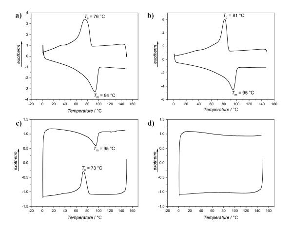
**Figure 27**: DSC analysis of the different approaches for the cleavage of **DP2**<sub>PE</sub> with ethylenediamine: **a)** Cleavage in DMF at 80 °C, **b)** cleavage in DMF at 80 °C, after direct addition of ethylenediamine to the decarboxylation mixture (one-pot two-step procedure, **c)** cleavage in 1,2,4-TCB at 80 °C and **d)** cleavage of PE-*b*-PEG with LiAlH<sub>4</sub>.
