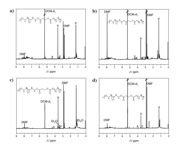
Figure 20: <sup>1</sup>H NMR spectra of PE-*b*-PEG (**DP2**<sub>PE</sub>) after photochemically-induced decarboxylation with **a**) reduced equivalents of phenylsilane, **b**) reduced concentration with respect to the polymer, **c**) additional *i*-PrOH and **d**) reduced concentration and additional *i*-PrOH. Solvent: DCM- $d_2$ .
