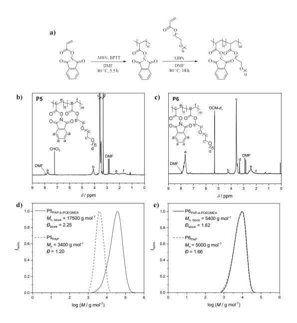
Figure 5: a) Synthesis of PAP-*b*-POEGMEA by chain extension of PAP *via* RAFT polymerization. b)<sup>1</sup>H NMR spectrum of P5. c) <sup>1</sup>H NMR spectrum of P6 and the corresponding SEC chromatograms in DMAc as eluent with PMMA calibration of d) P5 and e) P6.
