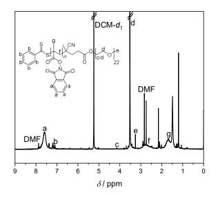
Figure 82: <sup>1</sup>H NMR spectrum of DPP1. Solvent: DCM-*d*<sub>2</sub>.
