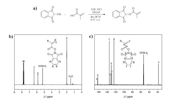
**Figure 43**: a) Synthesis of *N*-(methacryloyloxy)phthalimide (MAP) *via* Steglich esterification and analysis of the monomer by b) <sup>1</sup>H NMR spectroscopy and c) <sup>13</sup>C NMR spectroscopy in DCM- $d_2$  as solvent.
