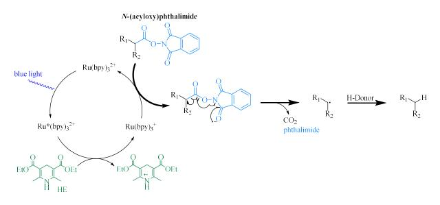
Scheme 20: Mechanism of the photochemical decarboxylation of the phthalimide activated ester *N*-(acyloxy)phthalimide as used in the present thesis with  $Ru(bpy)_3Cl_2$  as metal catalyst and HE (green) as reductant.<sup>113,115</sup>
