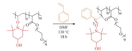
Scheme 48: Grafting styrene from PTEMVPO-*b*-POEGMEA by NMP upon heating to 130 °C.
