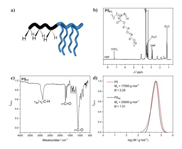
**Figure 7**: **a)** Schematic depiction of the block ratios of block copolymer P5<sub>PE</sub>, with PE (black) and POEGMEA (blue) blocks, as well as the analysis of P5<sub>PE</sub> via **b**) <sup>1</sup>H NMR spectroscopy, **c**) ATR-FT-IR spectroscopy, and the analysis of the block copolymers before and after decarboxylation by **d**) SEC with DMAc as eluent and PMMA calibration.
