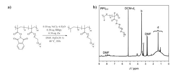
**Figure 49**: **a)** Thermal decarboxylation of **PP1** with NiCl<sub>2</sub>  $\cdot$  6 H<sub>2</sub>O, bbbpy and Zn in DMF/H<sub>2</sub>O (20:1) and **b)** the analysis *via* <sup>1</sup>H NMR spectroscopy.
