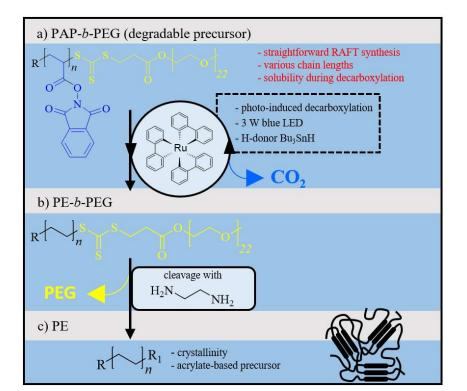
Scheme 35: Overview of the project idea to obtain pure PE from a) a soluble, degradable block copolymer which can be quantitatively decarboxylated to yield b) a degradable PE block copolymer which can be cleaved to yield c) PE.
