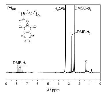
**Figure 55**: <sup>1</sup>H NMR spectrum of PAP (**P1**) after thermally-induced decarboxylation with tributyltin hydride in DMF/1,2,4-TCB (1:1) at 120 °C. Solvent: DMSO-*d*<sub>6</sub>, DMf-*d*<sub>7</sub>.
