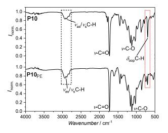
**Figure 15**: Comparison of the <sup>1</sup>H NMR spectra of **P10** (top) and **P10**<sub>PE</sub> (bottom). The removal of the  $\delta_{oop}$ C-H vibration is marked in red, while the arising signal of the C-H vibration of PE is marked in black.
