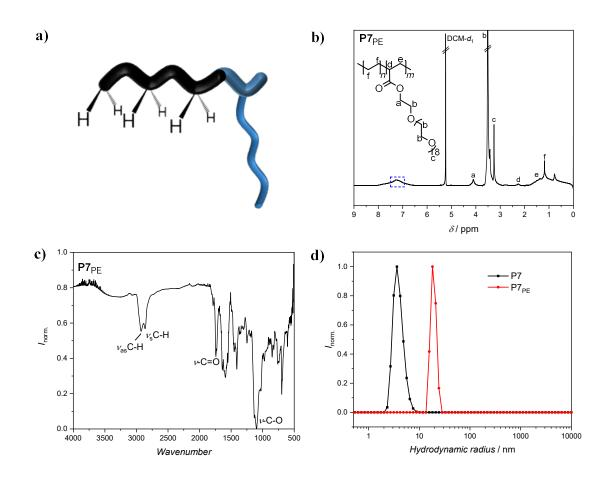
Figure 11: a) Schematic depiction of block ratios of block copolymer P7<sub>PE</sub>, with PE (black) and POEGMEA (blue) blocks, as well as the analysis of P7<sub>PE</sub> via b) <sup>1</sup>H NMR spectroscopy (additional, broad signal at 7.3 ppm marked in red), c) ATR-FT-IR spectroscopy, and the analysis of the block copolymers before and after decarboxylation by d) DLS.
