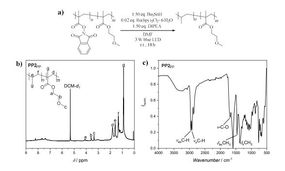
Figure 50: a) Decarboxylation of PP2 with  $Ru(bpy)_3Cl_2 \cdot 6 H_2O$ , DIPEA and  $Bu_3SnH$  as H-donor in DMF and the analysis of PP2<sub>PP</sub> via b) <sup>1</sup>H NMR and c) ATR-FT-IR spectroscopy.
