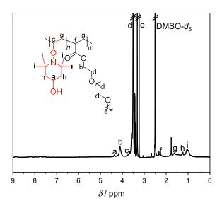
**Figure 79**: <sup>1</sup>H NMR spectrum of **PTEMVPO-***b***-POEGMEA** after reduction with Zn/AcOH in DMF at 60 °C; solvent: DMSO-*d*<sub>6</sub>.
