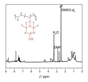
**Figure 78**: <sup>1</sup>H NMR spectrum of poly(ethylene-*co*-TEMVPO) after decarboxylation with  $Bu_3SnH$  and TEMPO-OH. Solvent: DMSO-*d*<sub>6</sub>.
