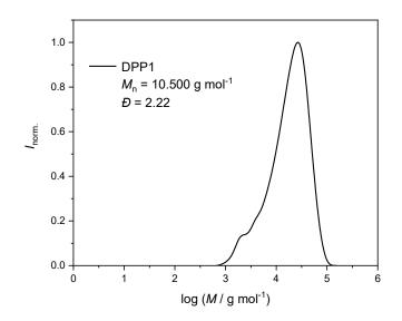
Figure 83: SEC chromatogram of DPP1 in DMAc as eluent and PMMA calibration.
