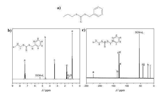
**Figure 4**: a) Structure of RAFT-agent *S*, *S'*- benzyl propyl trithiocarbonate (BPTT) and the analysis *via* b)  ${}^{1}$ H NMR and c)  ${}^{13}$ C NMR spectroscopy.
