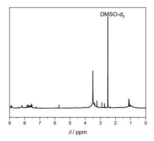
**Figure 88**: <sup>1</sup>H NMR spectrum of **PP1**<sub>PE</sub> after decarboxylation with Ru(bpy)<sub>3</sub>Cl<sub>2</sub> · 6 H<sub>2</sub>O, DIPEA and PhSiH<sub>3</sub> as H-donor. Solvent: DMSO- $d_6$ .
