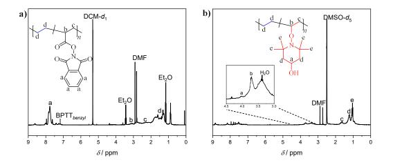
**Figure 38**: <sup>1</sup>H NMR spectra of the decarboxylation product **a**) after the first decarboxylation with Bu<sub>3</sub>SnH as H-donor, 0.50 eq. HE and 15 min reaction time and **b**) after the second decarboxylation with TEMPO-OH.
