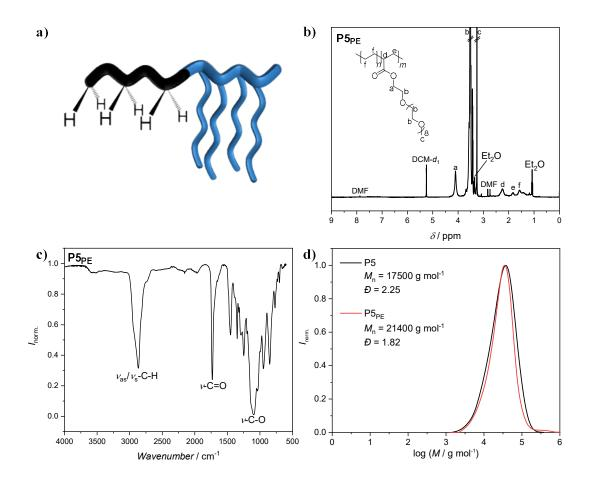
**Figure 8**: **a)** Schematic depiction of the block ratios of block copolymer P5<sub>PE</sub>, with PE (black) and POEGMEA (blue) blocks, as well as the analysis of P5<sub>PE</sub> via **b**) <sup>1</sup>H NMR spectroscopy, **c**) ATR-FT-IR spectroscopy, and the analysis of the block copolymers before and after decarboxylation by **d**) SEC with DMAc as eluent and PMMA calibration.
