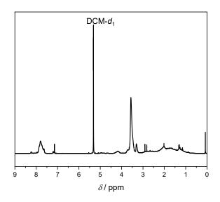
**Figure 87**: <sup>1</sup>H NMR spectrum of **PP1**<sub>PE</sub> after decarboxylation with Eosin Y as catalyst and DIPEA as H-donor. Solvent: DCM- $d_2$ .
