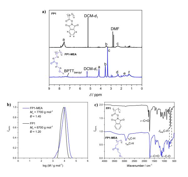
Figure 28: a) Comparison of the <sup>1</sup>H NMR spectra of PAP (FP1) (top, black) and after the Michael-type addition of MEA (FP1-MEA, bottom, blue); solvent: DCM- $d_2$ . b) SEC chromatogram of FP1 (black) and FP1-MEA (blue). c) Comparison of the ATR-FT-IR spectra of FP1 (top, black) and FP1-MEA (bottom, blue).
