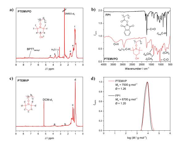
Figure 34: a) <sup>1</sup>H NMR spectrum of **PTEMVPO** after decarboxylation of PAP with TEMPO-OH; solvent: DMSO- $d_6$ . b) Comparison of ATR-FT-IR spectra of **FP1** (top, black) and **PTEMVPO** (bottom, red). c) <sup>1</sup>H NMR spectrum of **PTEMVP** after decarboxylation of PAP with TEMPO; solvent: DCM- $d_2$ . d) SEC chromatogram of **PTEMVP** and precursor **FP1** in DMAC as eluent with PMMA calibration.
