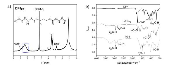
Figure 25: a) <sup>1</sup>H NMR spectrum of DP4<sub>PE</sub> after thermally-induced decarboxylation of DP4 with phenylsilane and b) analysis *via* ATR-FT-IR spectroscopy of DP4 (top, black), DP4<sub>PE</sub> (middle, grey) and PE4 (bottom, light grey).
