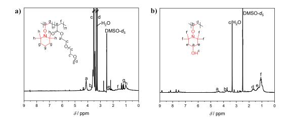
**Figure 41**: <sup>1</sup>H NMR spectra of the reduction of **a**) **PTEMVP-***b***-POEGMEA** in THF/H<sub>2</sub>O at 60 °C with Zn/AcOH followed by dialysis (Table 5, entry #6) and **b**) **PTEMVPO** in MeOH/THF/H<sub>2</sub>O at room temperature with Zn (Table 5, entry #9).
