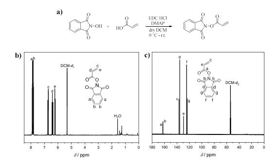
Figure 1: a) Synthesis of the monomer *N*-(acryloyloxy)phthalimide by Steglich esterification as well as the corresponding b) <sup>1</sup>H NMR and c) <sup>13</sup>C NMR spectrum.
