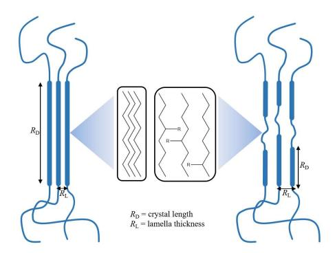
Scheme 34: Schematic depiction of the crystallinity of PE-*b*-POEGMEA after decarboxylation with H-donor Bu<sub>3</sub>SnH (left) and hindered crystallization of the PE block due to a small comonomer fraction after the decarboxylation with PhSiH<sub>3</sub> (right). Reduced crystal length ( $R_D$ ) and increased lamella thickness ( $R_L$ ) resulting in a decreased crystal size marked.
