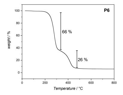
Figure 61: Thermogravimetrical analysis of P6, heating rate 10 K min<sup>-1</sup>.
