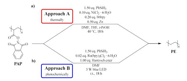
Scheme 27: a) Approach A: The thermal decarboxylation of the PAP homopolymer with phenylsilane as H-donor,  $NiCl_2 \cdot 6 H_2O$  and bbbpy as catalytic system and zinc as reductant. b) Approach B: The photochemical decarboxylation of the PAP homopolymer with phenylsilane as H-donor,  $Ru(bpy)_3Cl_2 \cdot 6 H_2O$  as catalytic system and HE as reductant.
