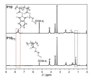
**Figure 14**: Comparison of the <sup>1</sup>H NMR spectra of **P10** (top) and **P10**<sub>PE</sub> (bottom). The removal of the aromatic proton signal is marked in red, while the arising signal of PE is marked in black.
