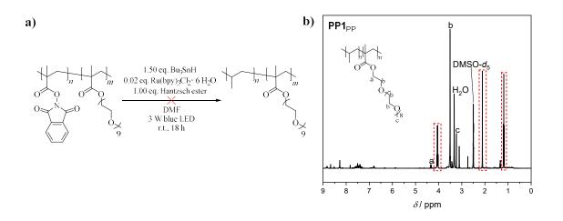
Figure 45: a) Decarboxylation of PP1 with  $Ru(bpy)_3Cl_2 \cdot 6 H_2O$ , HE and  $Bu_3SnH$  in DMF as solvent and b) the analysis of the resulting product *via* <sup>1</sup>H NMR spectroscopy.
