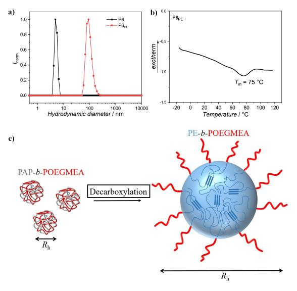
Figure 10: a) DLS analysis of PAP-*b*-POEGMEA (P6, black) and PE-*b*-POEGMEA (P6<sub>PE</sub>, red) after photochemically-induced decarboxylation as well as b) DSC characterization of P6<sub>PE</sub> after the addition of LiTFSI to favor the microphase separation and c) schematic depiction of the formation of agglomerates with partly crystalline PE in the core. As a result of the formation of agglomerates, the hydrodynamic radius  $R_h$  increases as demonstrated by DLS.
