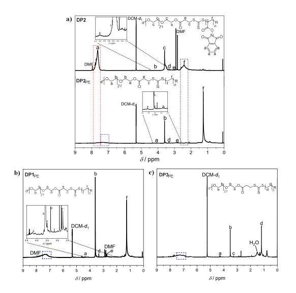
**Figure 18:** a) Comparison of the <sup>1</sup>H NMR spectra of **DP2** before (top) and after (**DP2**<sub>PE</sub>, bottom) the decarboxylation. b) <sup>1</sup>H NMR spectrum of **DP1**<sub>PE</sub>. c) <sup>1</sup>H NMR spectrum of **DP3**<sub>PE</sub>.
