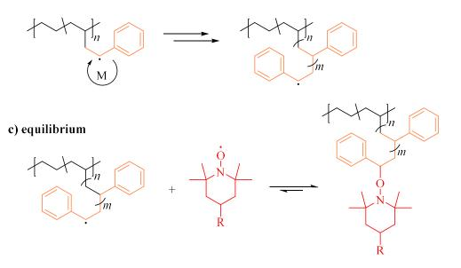
Scheme 15: The three main steps of the mechanism of grafting side chains from a TEMPOfunctionalized PE by NMP with a) the initiation upon heating to form the nitroxide and carboncentered radical which initiates the polymerization by reacting with the monomer, b) the propagation step, in which monomeric units are added to the side chain and c) the equilibrium between the propagating chain and the nitroxide with the stable alkoxyamine.
