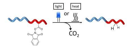
**Scheme 25**: Ethylene-free synthesis of PE block copolymers by either thermal or photochemical decarboxylation using an acrylate-based precursor polymer.
