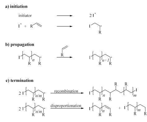
Scheme 1: Mechanism of free radical polymerization with three main steps: initiation, propagation, and termination.
