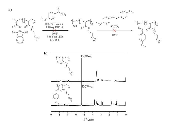
**Figure 33**: **a)** Decarboxylative thiolation with Eosin Y as the catalyst as used by Cao *et al.*<sup>134</sup> and **b)** the comparison of the <sup>1</sup>H NMR spectra of the first step (top) and the second step (bottom) of the reaction.
