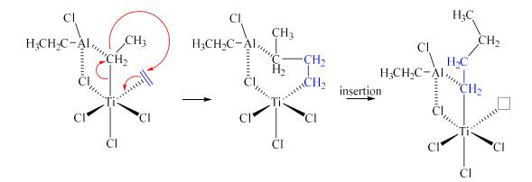
**Scheme 6**: Mechanism of the Ziegler-Natta process with the exemplary catalytic system TiCl<sub>4</sub> with diethylaluminiumchloride. **a**) Formation of the titanium-aluminium complex and the addition of the first ethylene unit (blue) to the free coordination position (grey box). **b**) Rearrangement of the electrons in the complex after addition of ethylene and insertion of ethylene into the titanium-carbon bond for the formation of a polymer chain.
