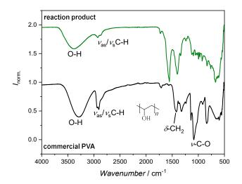
**Figure 39**: Comparison of the ATR-FT-IR spectra of the product after reduction of **PTEMVP** with Zn/AcOH in DMF (top, green) and of commercial PVA (black, bottom, Mowiol® 28-29,  $M_{\rm w} \sim 145.000$  g mol<sup>-1</sup>, Sigma-Aldrich).
