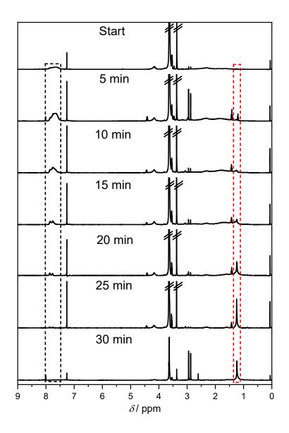
**Figure 64**: Reaction monitoring of photochemically-induced decarboxylation of PAP-*b*-POEGMEA (**P10**). Solvent: CDCl<sub>3</sub>.
