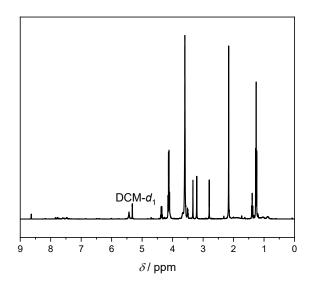
**Figure 85**: <sup>1</sup>H NMR spectrum of **PP1**<sub>PE</sub> after decarboxylation with  $Ru(bpy)_3Cl_2$  and HE as reductant and H-donor. Solvent: DCM- $d_2$ .
