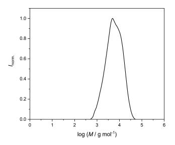
Figure 69: SEC chromatogram of PAP-BTTP-mPEG<sub>2000</sub> in DMAc as eluent with PMMA calibration.
