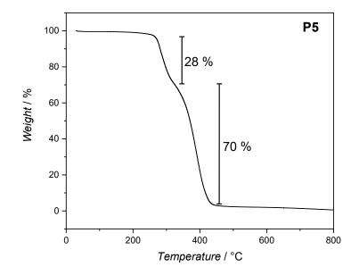
Figure 56: Thermogravimetrical analysis of P5, heating rate 10 K min<sup>-1</sup>.
