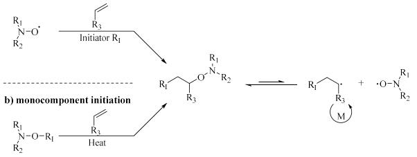
Scheme 2: Initiation of nitroxide-mediated polymerization by a) a bicomponent system with an initiator or b) by a monocomponent system with heat and the mechanism of NMP based on the equilibrium between dormant species (left) and the active species (right) with the propagating radical.
