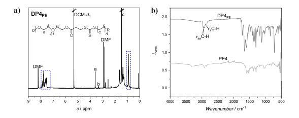
**Figure 26**: a) <sup>1</sup>H NMR spectrum of **DP4**<sub>PE</sub> after thermally-induced decarboxylation with Bu<sub>3</sub>SnH and the corresponding b) comparison of the ATR-FT-IR spectra of **DP4**<sub>PE</sub> and **PE4**.
