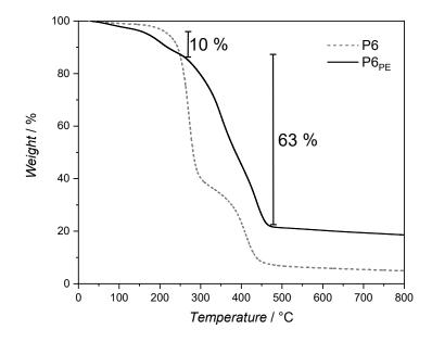
Figure 62: Thermogravimetrical analysis of  $P6_{PE}$  in comparison to P6, heating rate 10 K min<sup>-1</sup>.
