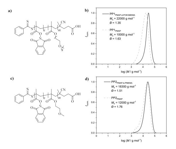
**Figure 44**: **a)** Structure of PMAP-*b*-POEGMEMA (**PP1**) polymerized by RAFT polymerization with 4-cyano-4-((phenylcarbonothioyl)thio)pentanoic acid (CTP). **b)** SEC chromatogram of PMAP (grey, dashed) and PMAP-*b*-POEGMEMA (**PP1**, black) in DMAc as eluent with PMMA calibration. **c)** Structure of PMAP-*b*-PMEMA (**PP2**) and **d)** SEC chromatogram of PMAP (grey, dashed) and PMAP-*b*-PMEMA (**PP2**, black) in DMAc as eluent with PMMA calibration.
