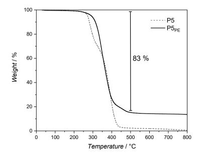
Figure 57: Thermogravimetrical analysis of  $P5_{PE}$  in comparison to P5, heating rate 10 K min<sup>-1</sup>.
