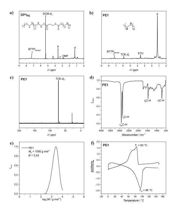
Figure 24: a) <sup>1</sup>H NMR spectrum of PE-*b*-PEG (DP1), solvent: DCM- $d_2$ . Analysis of PE1 *via* b) HT-<sup>1</sup>H NMR spectroscopy, benzyl end group and ETU marked, solvent: TCE- $d_2$ , c) HT-<sup>13</sup>C NMR spectroscopy, solvent: TCE- $d_2$ , d) ATR-FT-IR spectroscopy, e) HT-SEC in 1,2,4-TCB at 160 °C and f) DSC.
