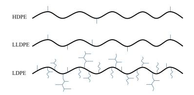
**Scheme 9**: Presentation of the molecular structure of different types of PE: rarely branched high-density PE (HDPE), slightly branched linear low-density PE (LLDPE) and highly branched low-density PE (LDPE).
