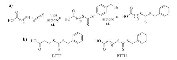
Scheme 36: a) Synthesis of the basic structure of the RAFT agents and b) detailed structure of the RAFT agents 3-(((benzylthio)carbonothioyl)thio)propanoic acid (BTTP) and 11-(((benzylthio)carbonothioyl)thio)undecanoic acid (BTTU) evaluated for the synthesis of the degradable PAP block copolymers.
