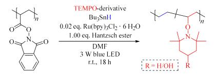
**Scheme 45**: Synthesis of poly(ethylene-*co*-TEMVP) from PAP by simultaneous decarboxylation with TEMPO/TEMPO-OH and Bu<sub>3</sub>SnH as H-donor.
