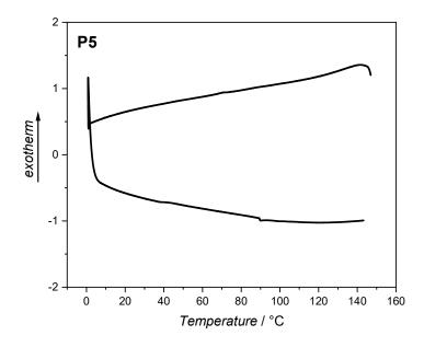
Figure 58: DSC characterization of P5, heating rate 10 K min<sup>-1</sup>.
