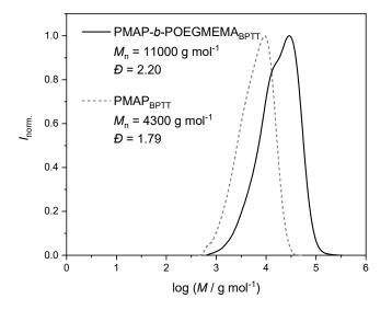
**Figure 81**: SEC chromatogram of PMAP (grey, dashed) and PMAP-*b*-POEGMEMA (black) polymerized with BPTT as RAFT agent in DMAc as eluent with PMMA calibration.
