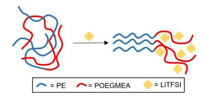
**Scheme 32**: Schematic depiction of the effect of the LiTFSI addition The salt accumulates exclusively in the POEGMEA phase, increasing the microphase separation and thus enables the crystallization of PE.
