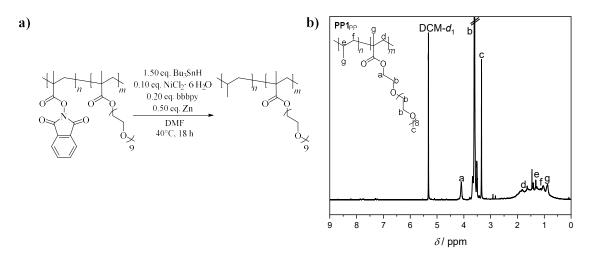
**Figure 48**: **a)** Thermal decarboxylation of **PP1** with NiCl<sub>2</sub>  $\cdot$  6 H<sub>2</sub>O, bbbpy, Zn and Bu<sub>3</sub>SnH as H-donor in DMF and **b)** the analysis *via* <sup>1</sup>H NMR spectroscopy.
