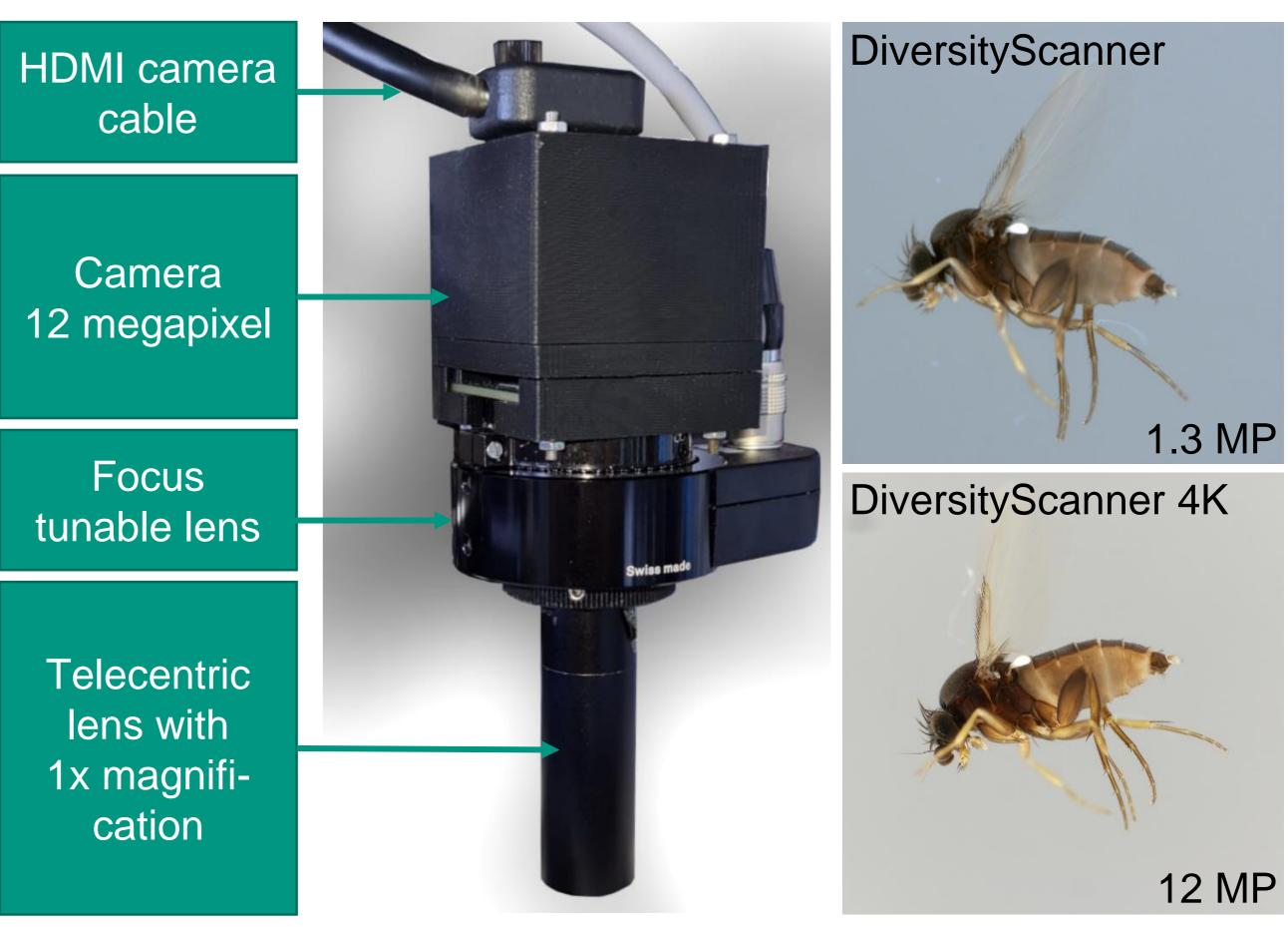
High resolution (12 MP) camera with a small pixel size  $(1.55 \ \mu m \ x \ 1.55 \ \mu m)$  for very sharp images and focus tunable lens (Optotune, Switzerland) for focus stacking
