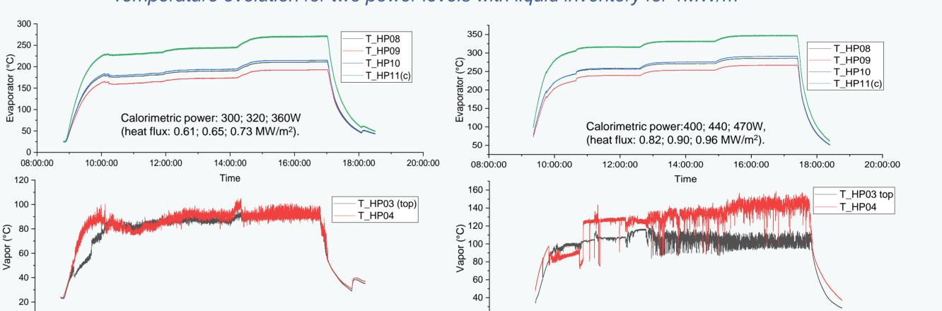
Temperature evolution for two power levels with liquid inventory for 1MW/m<sup>2</sup>
