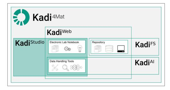
Figure 4 Conceptual overview of Kadi4Mat. Currently two software modules are available: (1) KadiWeb, a web-based virtual research environment incorporating ELN functionalities and repositories and (2) KadiStudio, a desktop-based software version which allows for the formulation and execution of workflows. Further modules such as a machine learning implementation referred to as KadiAI and a desktopbased repository called KadiFS are subject of current developments.
