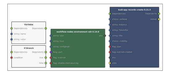
Figure 6 Available node types. Built-in nodes are grey, environment nodes green and tool nodes blue.
