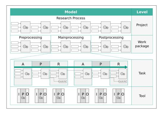
Figure 2 Abstraction of a research process at different levels of detail. Each grey box with gears models a work step while the white boxes represent their parameterisation. APR refers to the description of tasks as data acquisition, data processing, and data routing. Iteratively structuring a research process according to the IPO model ultimately defines it via multiple generic tools.
