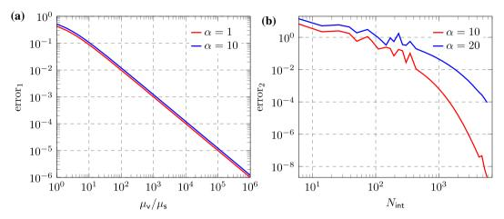
Fig. 7 Error measure error<sub>1</sub>( $\mu_v/\mu_s, \alpha$ ) addressing the issue of approximating the incompressible limit  $\mu_v/\mu_s \rightarrow \infty$  by finite  $\mu_v/\mu_s$  regarding the viscous polarization tensor in (a) and error measure error<sub>2</sub>( $N_{int}, \alpha$ ) addressing the numerical integration of the polarization tensor regarding the number of integration points  $N_{int}$  in (b)
