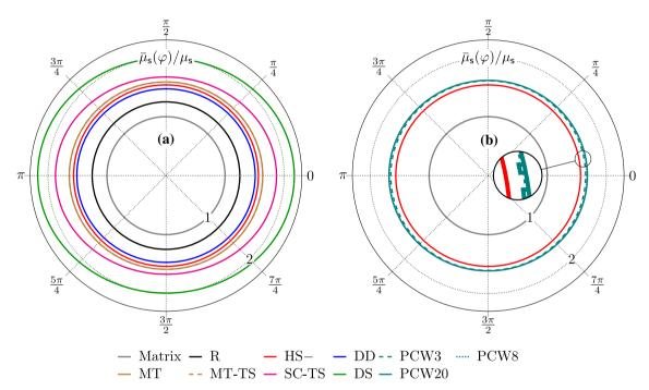
**Fig. 3** Dimensionless effective shear viscosity of a fiber suspension in the  $e_1$ - $e_2$ -plane: Results regarding classical mean-field models shown in (**a**) and results regarding PCW shown in (**b**) (orientation state and settings given in Sect. 7.1)
