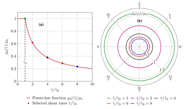
Fig. 9 Power-law function  $\mu_{s}(\dot{\gamma}/\dot{\gamma}_{0})/\mu_{s}$  representing the shear thinning matrix behavior given in (a) and effective viscosity  $\bar{\mu}_{s}(\varphi, \dot{\gamma}/\dot{\gamma}_{0})/\mu_{s}$  for selected shear rates with respect to MT given in (b)
