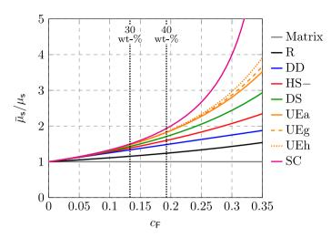
Fig. 8 Normalized effective shear viscosity for the special case of spherical inclusions with respect to different mean-field models and fiber volume fraction
