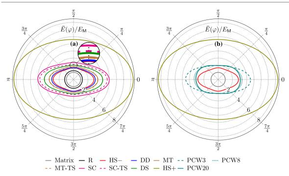
Fig. 5 Dimensionless effective Young's modulus of a fiber reinforced composite in the  $e_1$ - $e_2$ -plane: Results regarding classical mean-field models shown in (a) and results regarding PCW shown in (b) (orientation state and settings given in Sect. 7.1)
