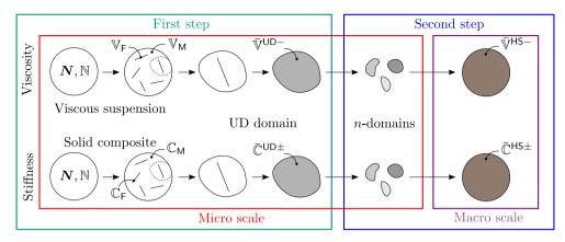
Fig. 1 Hashin–Shtrikman two-step procedure for the lower bound of viscous fiber suspensions and for the lower/upper bounds of solid fiber reinforced composites (own sketch based on Kehrer et al. [47])
