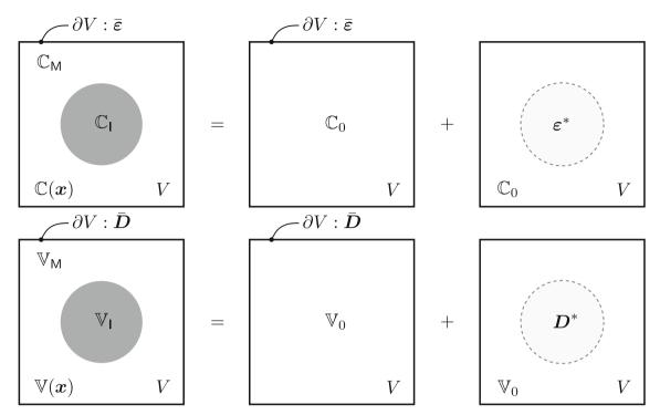
Fig. 6 Principle of equivalent eigenstrain (upper part) and principle of equivalent eigenstrain rate (lower part) to consider inhomogeneities embedded in a matrix (own sketch based on Gross and Seelig [14] and Brylka [43])
