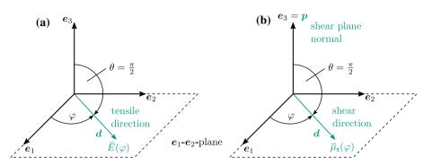
Fig. 2 Visualization procedure regarding the direction-dependent effective Young's modulus shown in (a) and regarding the effective shear viscosity shown in (b), restricted to the  $e_1$ - $e_2$ -plane ( $\theta = \pi/2$ ) parameterized by  $\varphi \in [0, 2\pi)$
