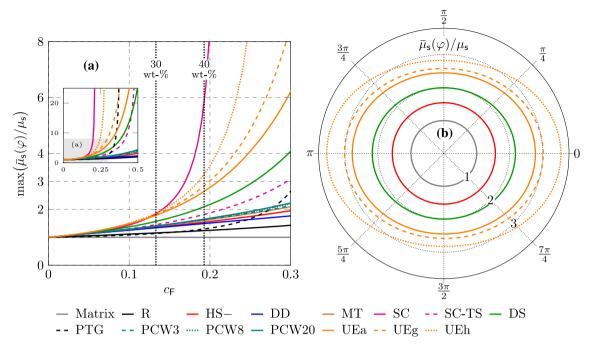
Fig. 4 Dimensionless effective shear viscosity of a fiber suspension in the  $e_1$ - $e_2$ -plane: Maximum viscosity for SC, SC-TS, DS shown in (a) and viscous anisotropy based on the upper estimates shown in (b) (orientation state and settings given in Sect. 7.1)
