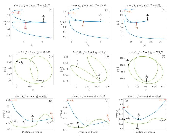
FIG. 7: Branches show intracavity power  $||u||_2^2 = \frac{1}{2\pi} \int_0^{2\pi} |u(s)|^2 ds$  of the soliton u plotted vs. values of  $\zeta_0$  or  $\omega$ . First row: blue branch as achieved by the first  $\zeta_0$ -optimization. Second row: green branch as achieved by the first  $\omega$ -optimization. Third row: FWHM along these branches. Columns correspond to different values of d,  $f_1$ , f.
