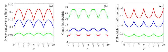
FIG. 2: Power conversion efficiency, comb bandwidth and full-width at half-maximum as a function of  $\varphi$  for three different examples. The blue curves correspond to d=0.1 and f=2, the red ones to d=0.25 and f=2 as well as the green ones to d=0.1 and f=5.
