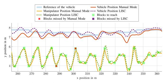
Fig. 6: Trajectories of the 5th test subject in manual mode and with the proposed LISC.
