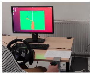
Fig. 3: An image of the test-bench with the GUI, steering wheel and joystick (bottom right).
