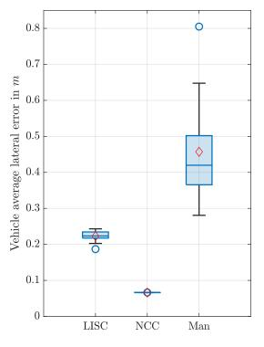
Fig. 5: Box plot of the average vehicle errors and deviations for the three different control modes (LISC, NCC, manual)
