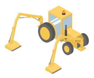
Fig. 1: An example of a large vehicle-manipulator: Two hydraulic actuated manipulators are attached to a tractor.
