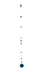
Fig. 6. Satellite drops in inkjet printing. The main droplet is followed by multiple smaller droplets.
