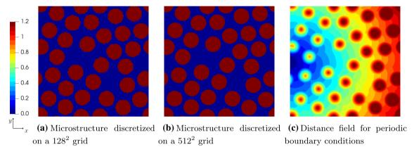
Fig. 8 Microstructure containing 32 circular inclusions for different resolutions and distance field for periodic boundary conditions
