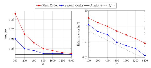
(a) Effective crack energy vs. number of pixels per di- (b) Relative error of the effective crack energy vs number mension of pixels per dimension
