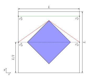
**Fig. 4** Example for (non-unique) shortests path with Dirichlet (index "D", red) and periodic (index "P", green) boundary conditions
