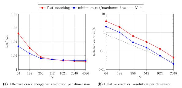
Fig. 10 Effective crack energy and relative error comparing fast marching with minimum cut/maximum flow
