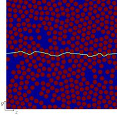
**(b)** Crack path for Dirichlet boundary conditions at  $x_2 = L/2$
