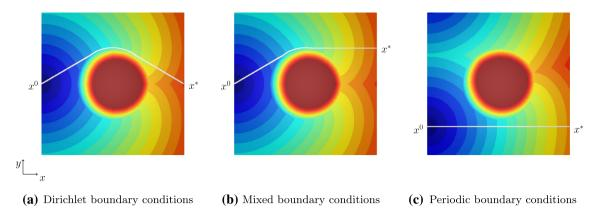
Fig. 5 Distance field and crack path for different boundary conditions for a single circular inclusion microstructure
