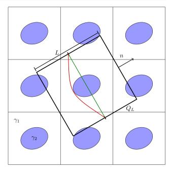
**Fig. 1** Visualization of the computation of the effective crack energy. The cube  $Q_L(n)$  is placed into the periodic structure. Depending on the material contrast  $\gamma_2/\gamma_1$  either the green or the red path is favored
