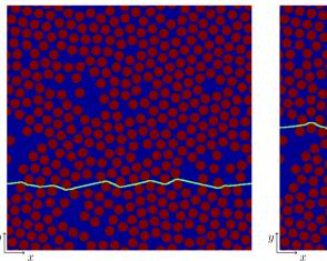
(a) Absolute minimum crack path - periodic boundary conditions
