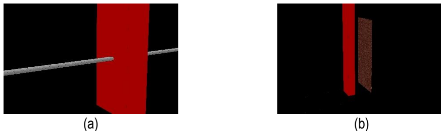
Figure 1.2 – a ) Hard clash between a pipe and a beam; b ) Soft clash between a door and a beam.
