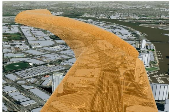
Figure 2.7 – a) Noise influence area for different noise sources (adapted from Melbourne Planning Scheme Ordinance, p. 1281); b) noise impact regulation in 3D using sweeping
