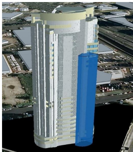
Figure 2.4 – Overlooking regulation in 3D using CSG
