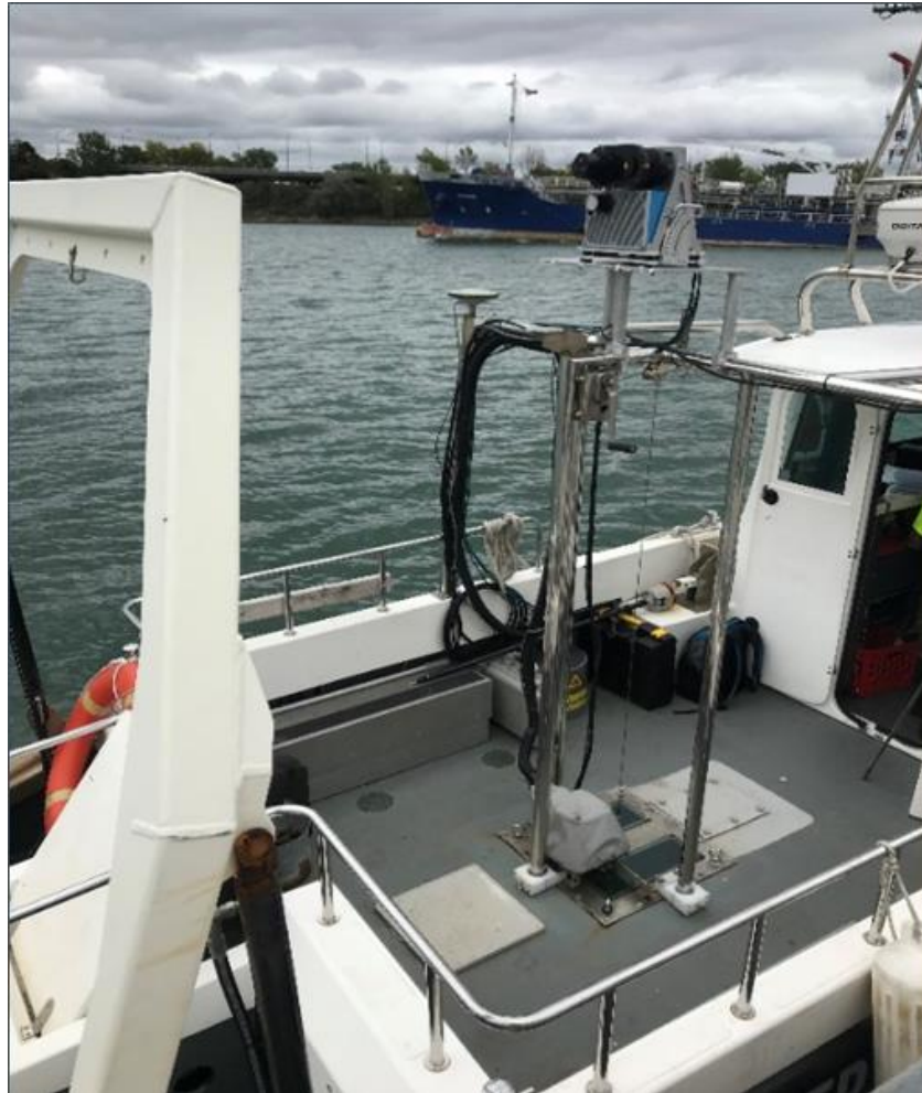
Figure 1.11 – Mobile LiDAR system mounted on a hydrographic vessel (Courtesy of CIDCO)
