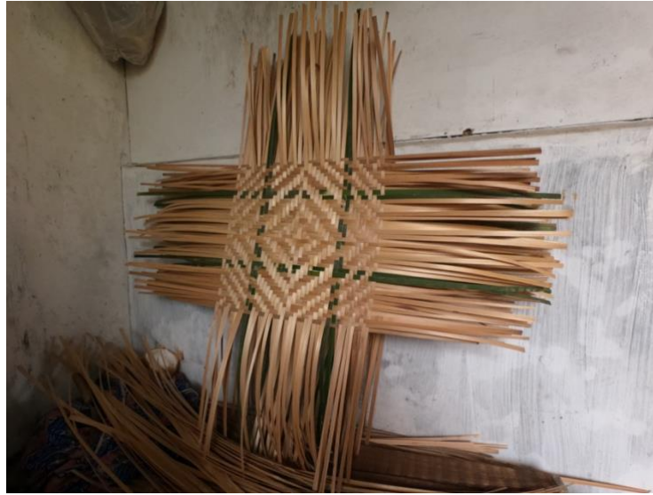
Figure 20 The woven base of tolombong ( tolok ) that are collected before the forming process ( dipengkorkeun ).
