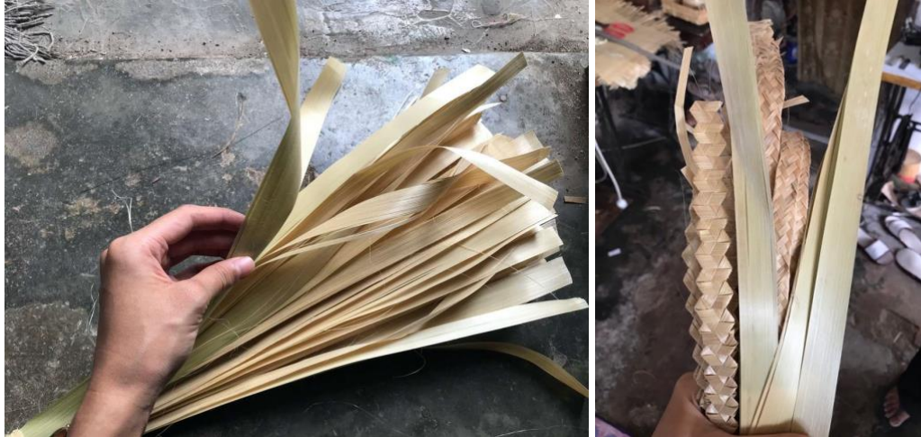
Figure 52 Raw-thin-sliced bamboo material (left); woven ropes (right) for fine woven bamboo crafts (Parhon's trademark).
