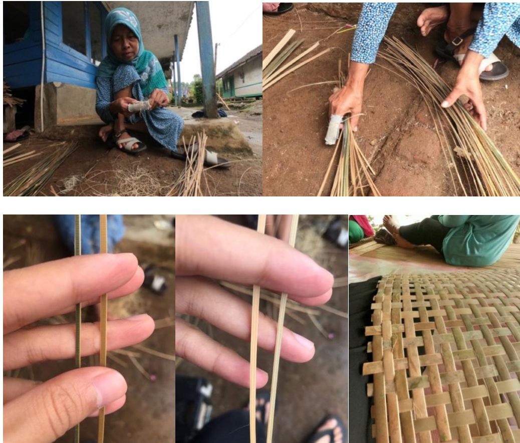
Figure 24 Processing bamboo strips for producing ayakan . Left to right, first row: shaping the sides of strips; collecting the finished strips. Left to right, second row: the outer layer of bamboo (inner part, green and yellowish colors); the inner part of the outer layer of bamboo; woven strips for (big-sized) ayakan .
