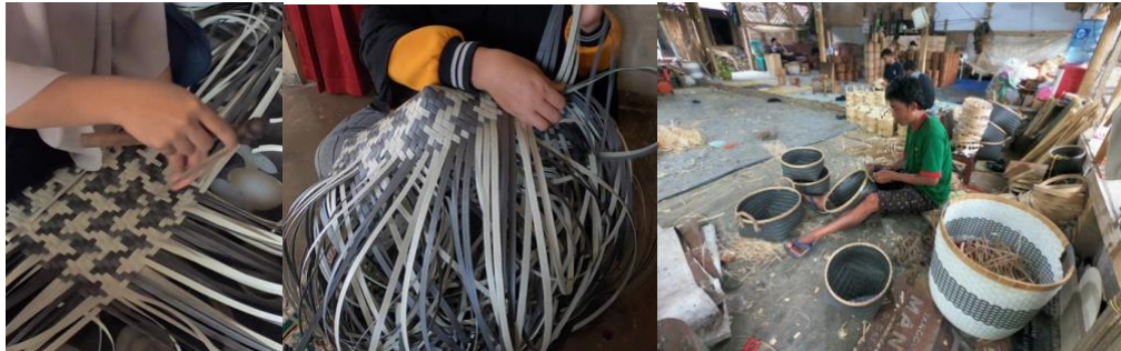
Figure 44 Producing processes with artificial materials: weaving process (left) was done by weavers nearby; the framing and finishing process (right) was done in the central workshop.
