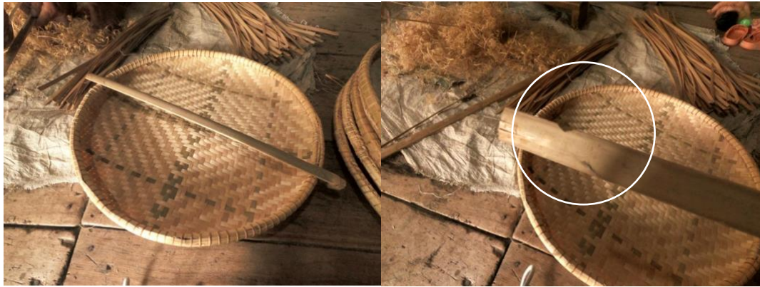
Figure 23 Manual measurement made of bamboo stick to make nyiru .
