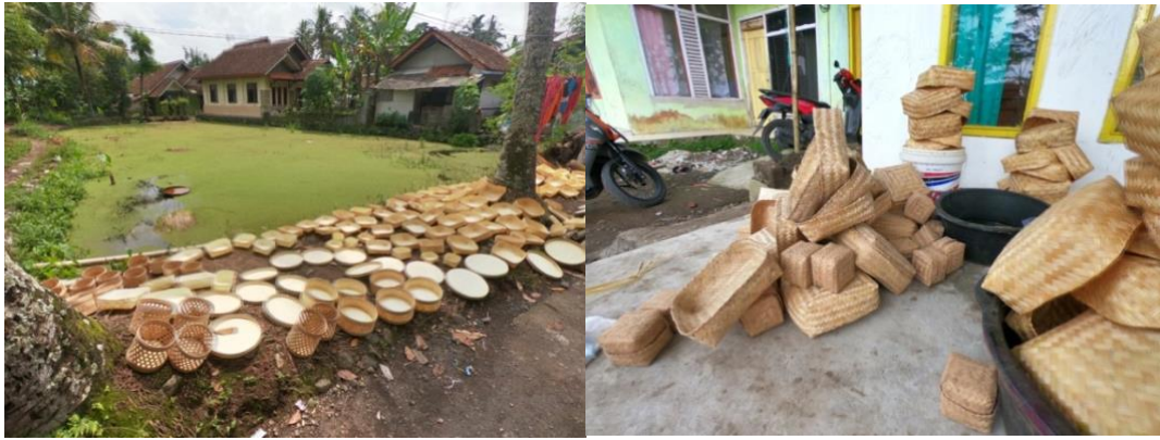
Figure 43 The process of dip, drain, and dry the finished woven bamboo products to the preservative and whitening liquids.
