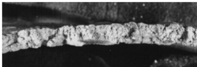
FIG. 4. Macroscopic Picture of Cracked Weld Joint
