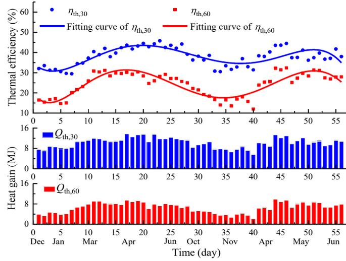
Fig. 7. Thermal performance of the a-Si PV/T systems at 30 °C and 60 °C.
