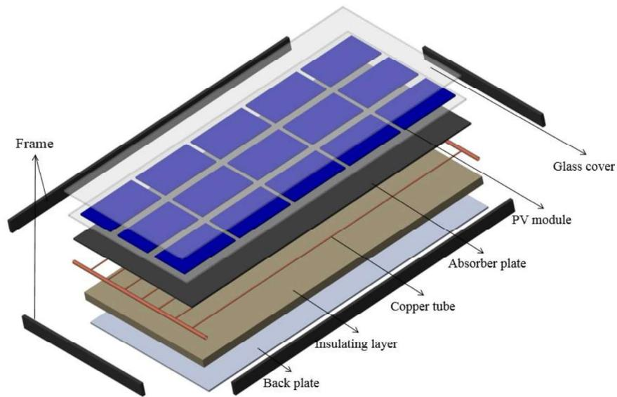
Fig. 3 Structure of the a-Si PV/T collector.
