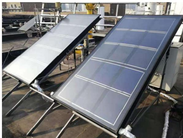
Fig. 4. Actual setup of two a-Si PV/T systems.
