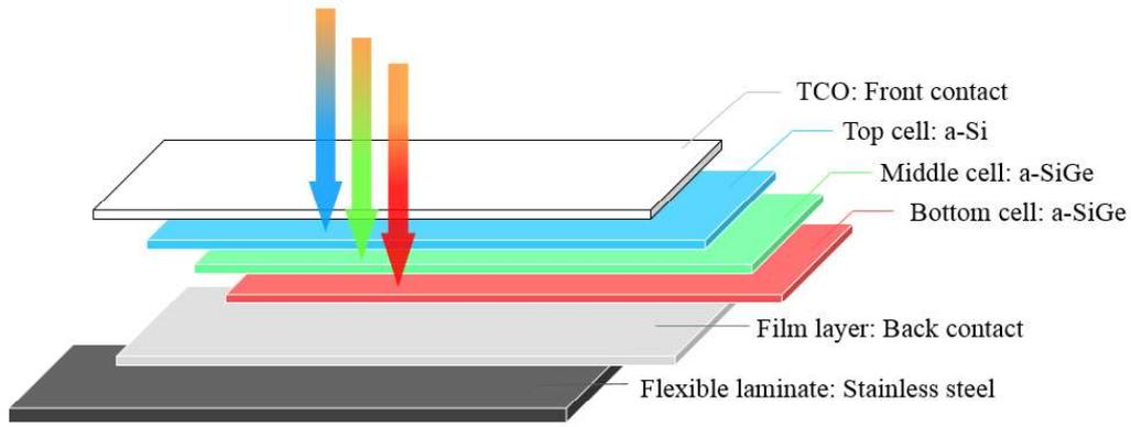
Fig. 1 Structure of the triple-junction a-Si cells.
