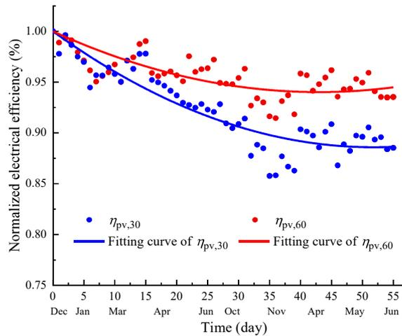
Fig. 10. The normalized electrical efficiency of the a-Si PV/T systems at 30 °C and 60 °C.
