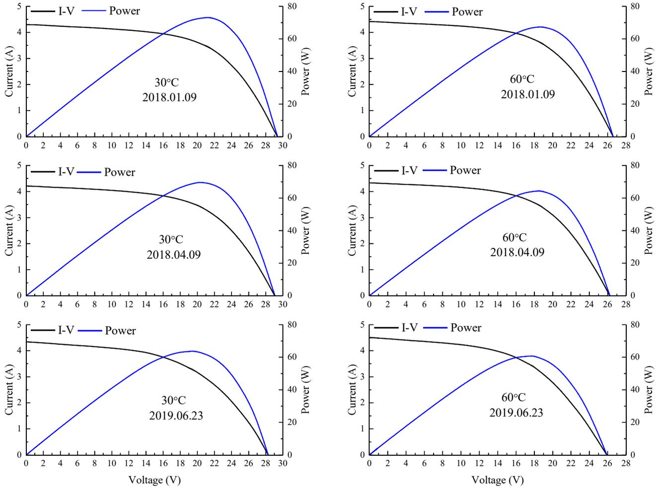
Fig. 17. I-V characteristics curve of the a-Si PV/T systems operating at 30 °C and 60 °C.
