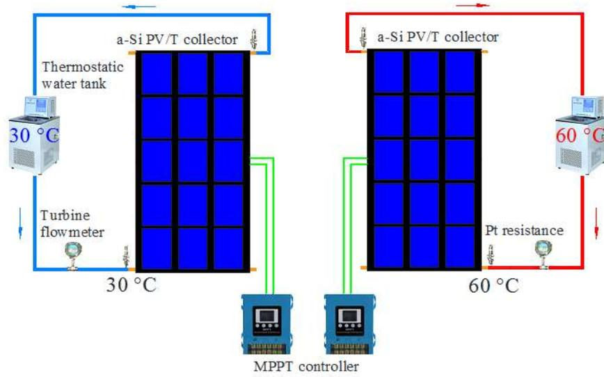
Fig. 5. Schematic diagram of two a-Si PV/T systems.
