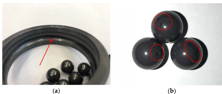
Figure 12. Outer ring raceway and rolling bodies of full ceramic ball bearing after the test. (a) Bearing outer ring raceway, (b) Rolling bodies.
